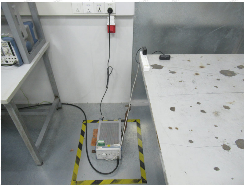
Photo of Conducted Emission Measurement
