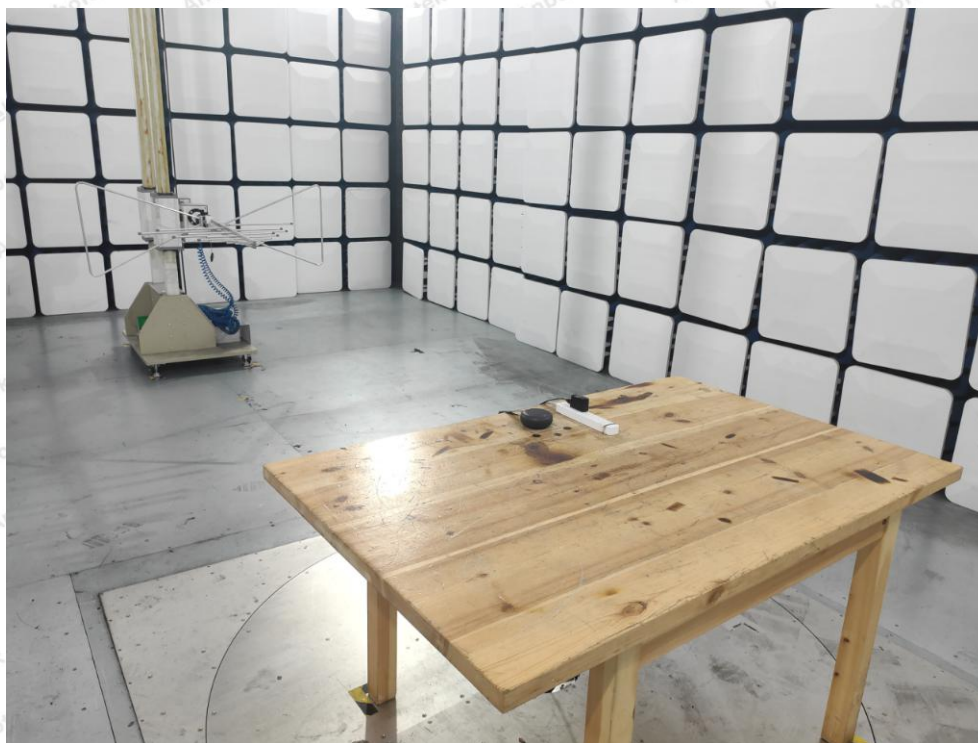
Photo of Radiation Emission Test
