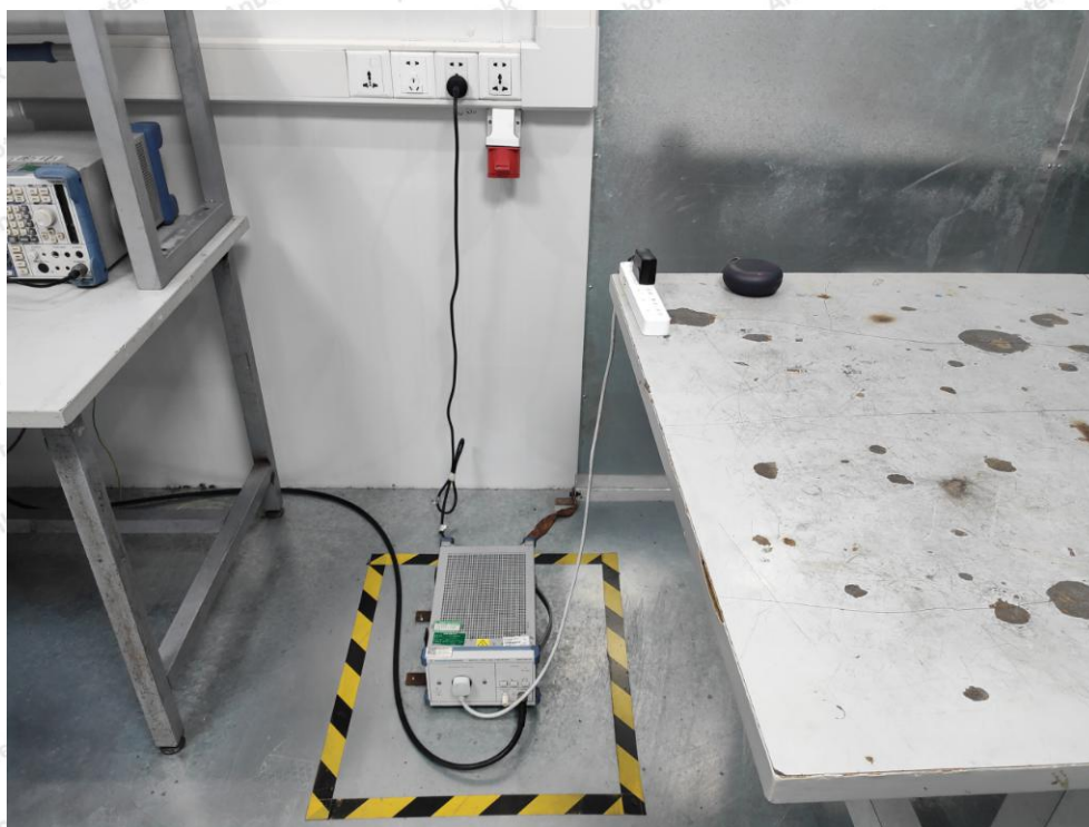
Photo of Conducted Emission Measurement
