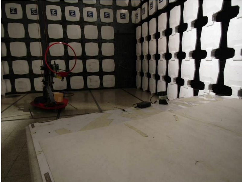
Measurement of Radiated Emission Test Set Up (30MHz – 1000MHz)
