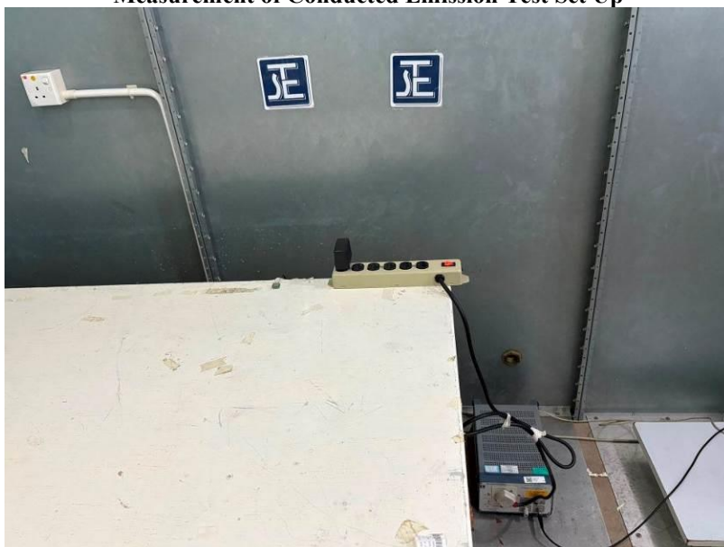
Measurement of Conducted Emission Test Set Up
