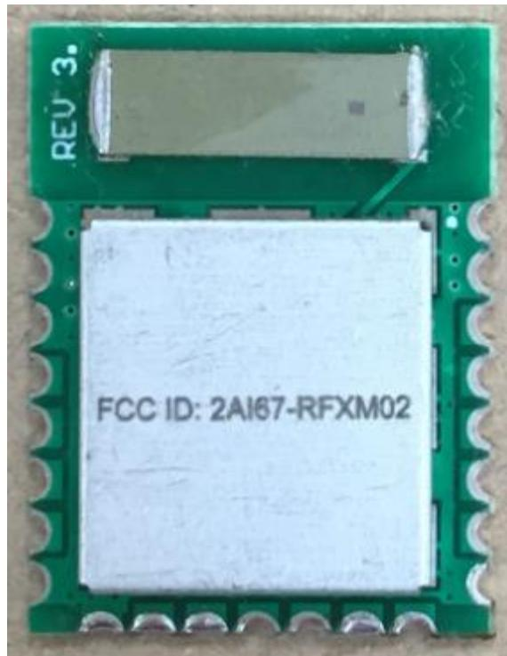
TMWRFX-M-CHIP is a wireless module. Design based on TI CC1310 high-performance wireless transceiver chip, is a two-way wireless receiving and transmitting module, Wireless frequency is 433.92MHZ.
