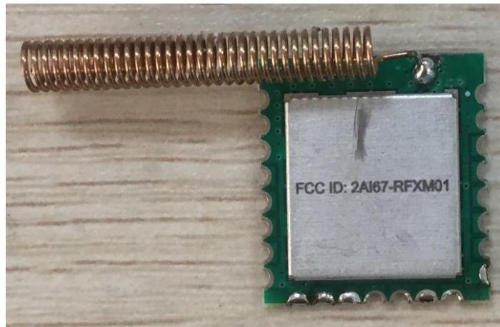
TMWRFX-M-COIL is a wireless module. Design based on TI CC1310 high-performance wireless transceiver chip, is a two-way wireless receiving and transmitting module, Wireless frequency is 433.92MHZ.
