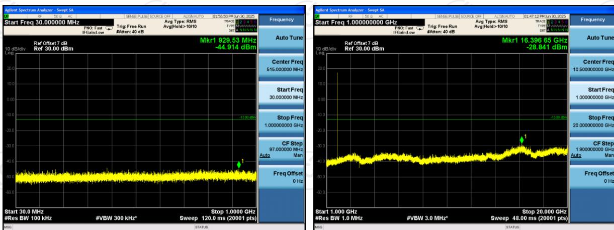
Conducted Spurious Emission on Channel 9400
