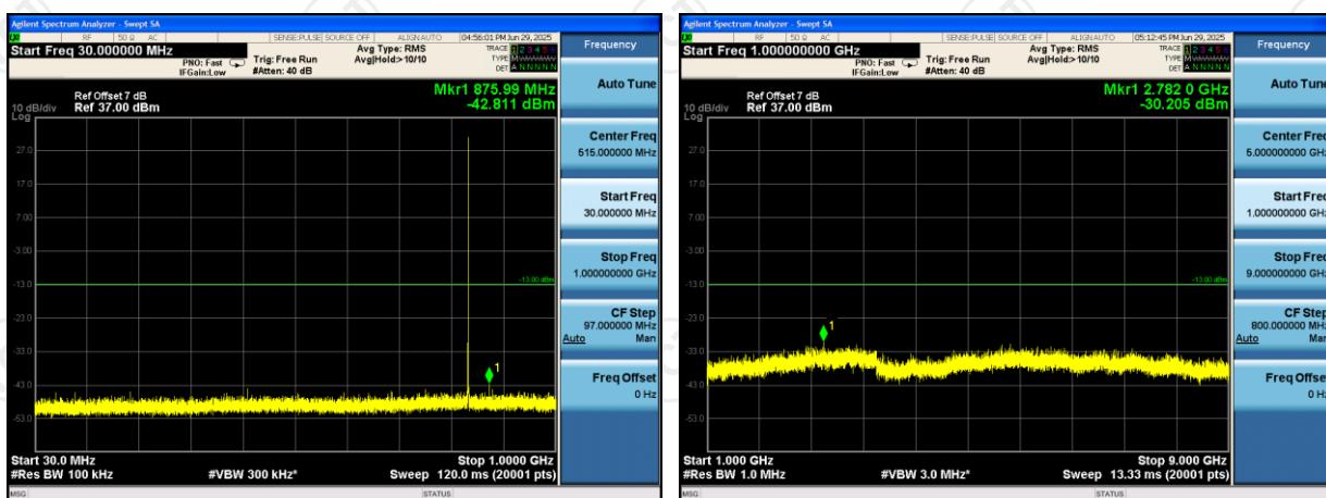
Conducted Spurious Emission on Channel 251
