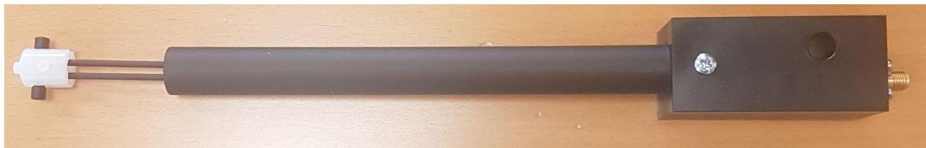
**Figure 1 – MVG COMOSAR Validation Dipole**
