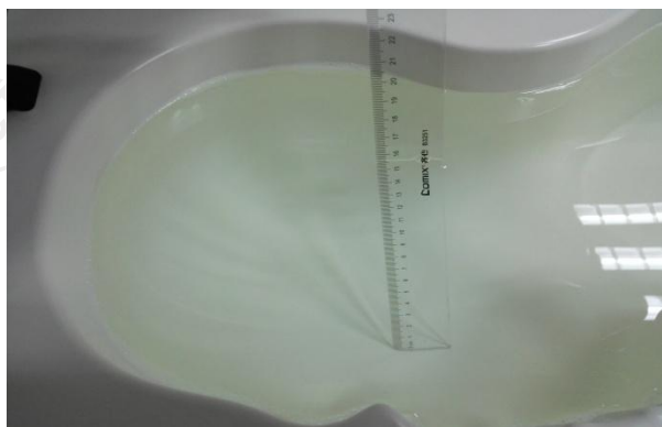
The Head Liquid of 1900MHz (15.5cm)
