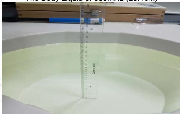
The Body Liquid of 1900MHz (16.4 cm)
