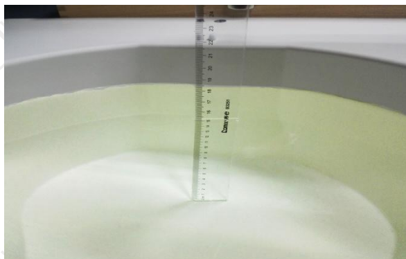
The Body Liquid of 1800MHz (15.2 cm)
