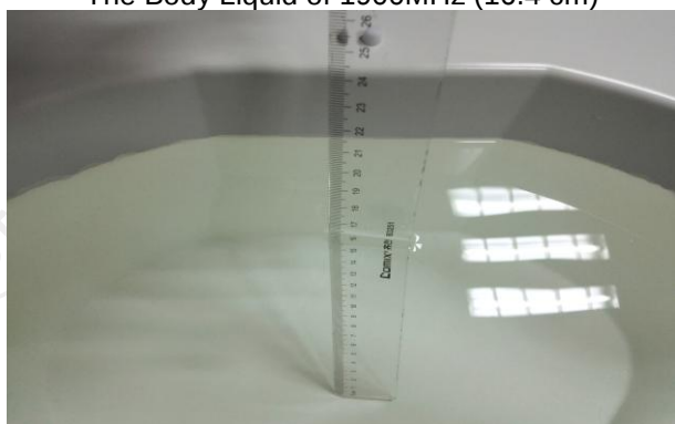
The Body Liquid of 2600MHz (16.5cm)
