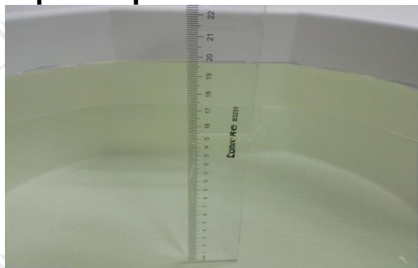
The Body Liquid of 835MHz (15.4cm)
