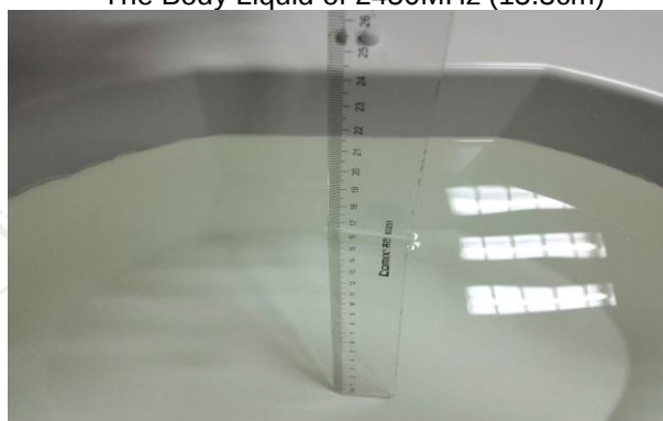
The Body Liquid of 5000-6000MHz (16.5cm)
