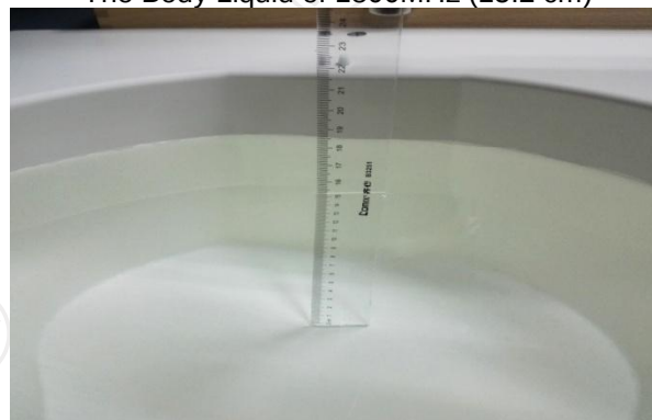
The Body Liquid of 2450MHz (15.3cm)
