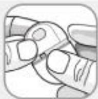
Align the holes on the patch with the main unit's sensor probe, adhere it, and press firmly.
