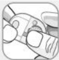
Replace it with a new battery (CR1216), ensuring the correct orientation with the "+" symbol facing upward as indicated on the product.
