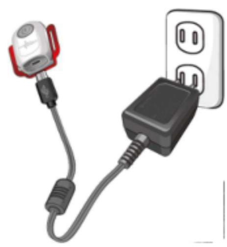
Before first use (around 2 hours). Plug the Type-C end of the charging adaptor into the charging port on the Infant Oximeter Box. The charging LED will turn off when fully charged.
