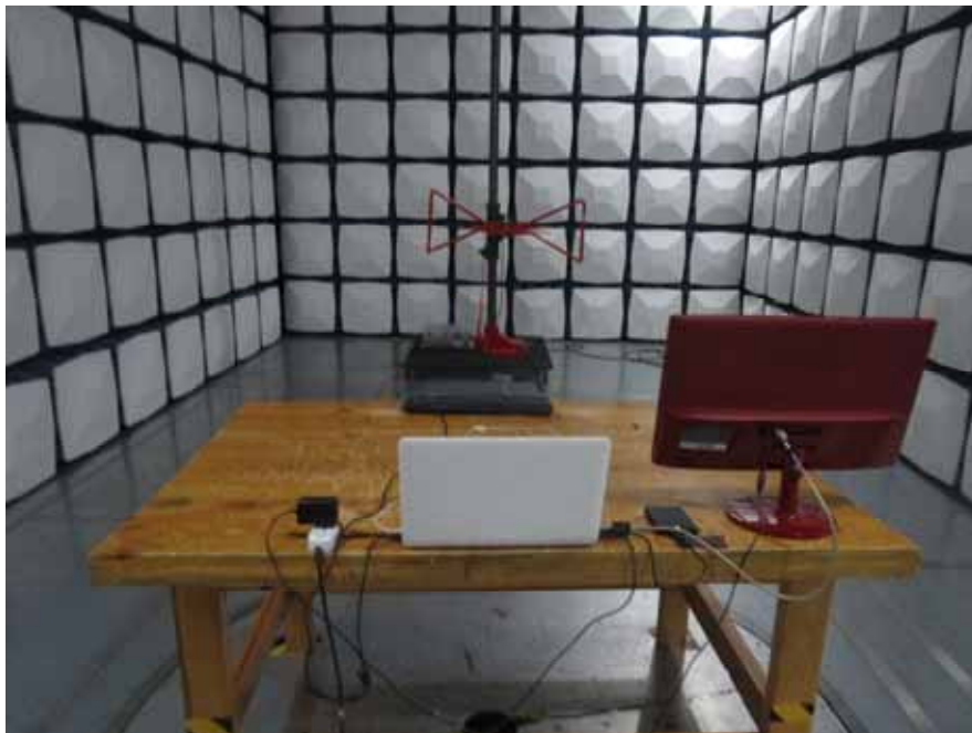
Radiated Emissions – Rear View (Below 1GHz) (Adapter#1)
