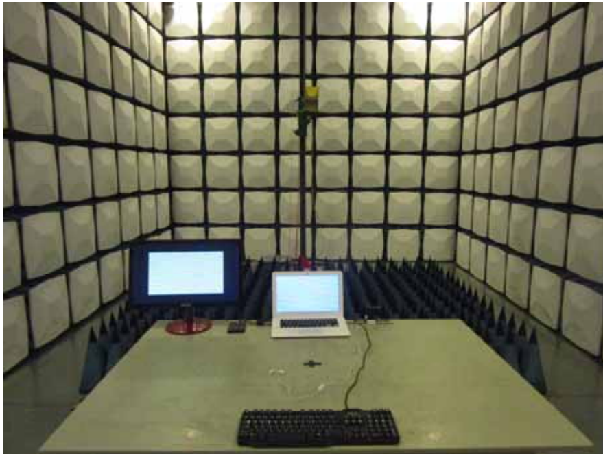
Radiated Emission – Front View (Above 1 GHz) (Adapter#1)
