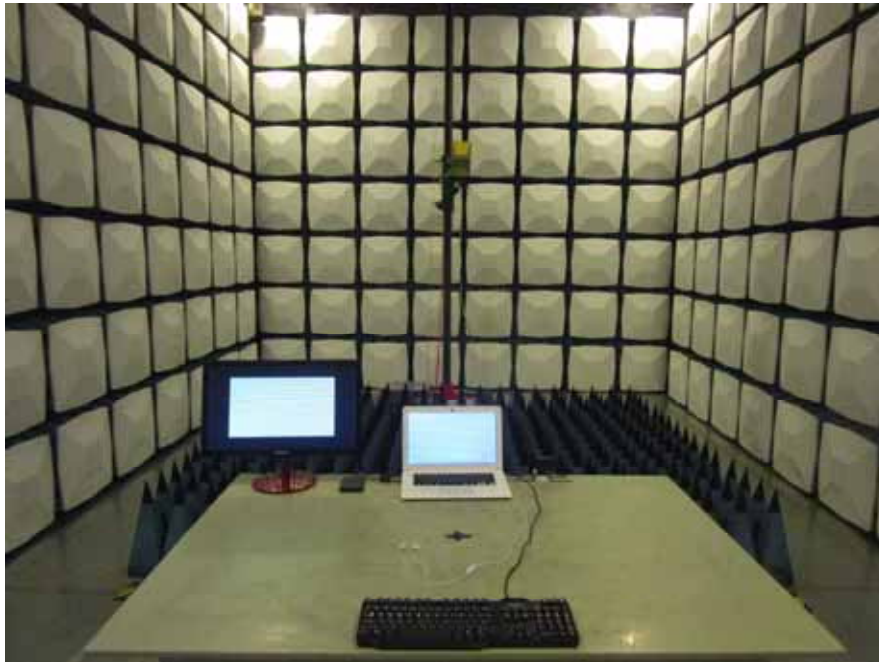
Radiated Emission – Front View (Above 1 GHz) (Adapter#2)
