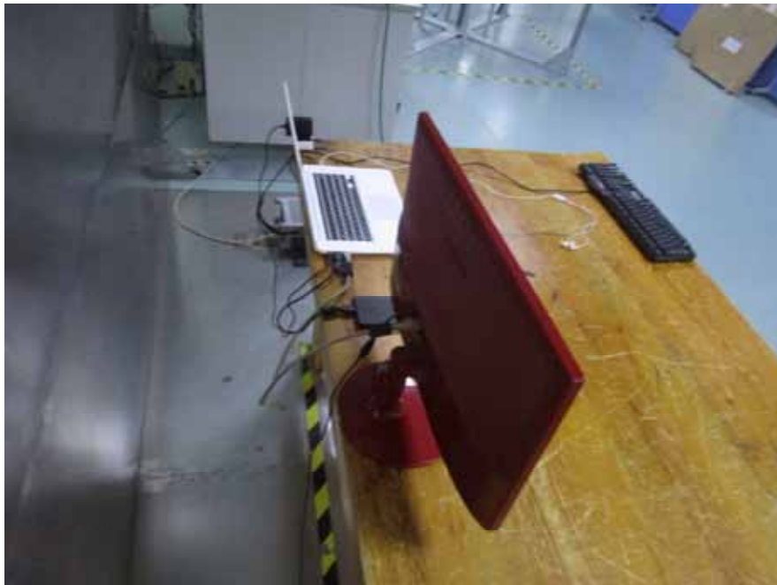
Conducted Emissions - Side View (Adapter#1)
