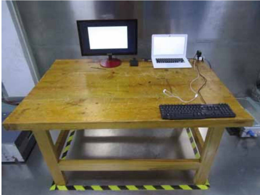
Conducted Emissions – Front View (Adapter#1)
