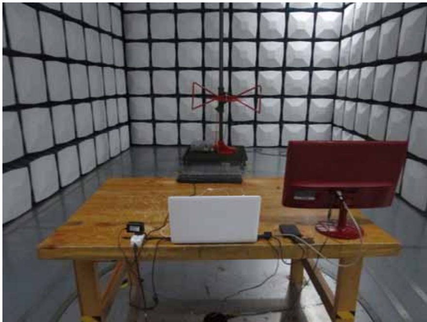
Radiated Emissions – Rear View (Below 1GHz) (Adapter#2)
