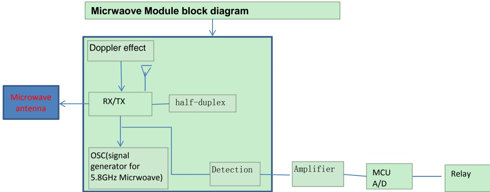
OSC emits a signal at a high frequency 5.8GHz and receives its echo, if a movement in the detection zone changes the echo, the echo signal will be amplified and sent to MCU. MCU processes the signal as high-low-level to control relay.
