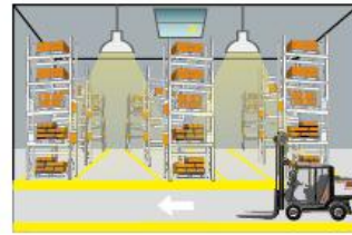
③ After hold time, the lamp gradually dims to a low light level 10% if no movement detected.
