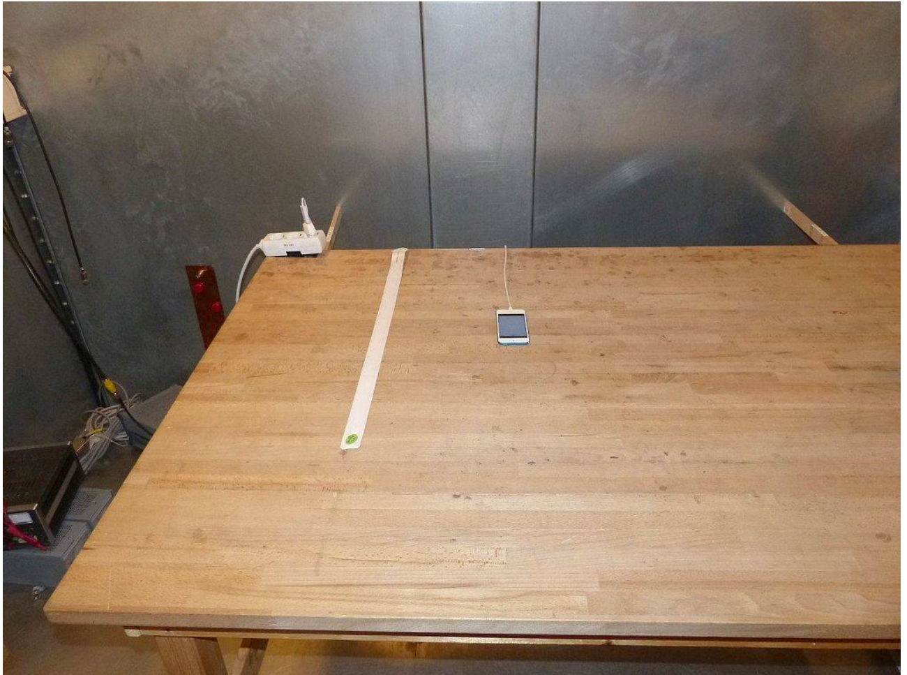
Photo 6: Test setup for conducted measurements (AC Port (power line), EUT supplied by AC/DC adapter, unintentional radiator §15.107, ANSI C63.4)
