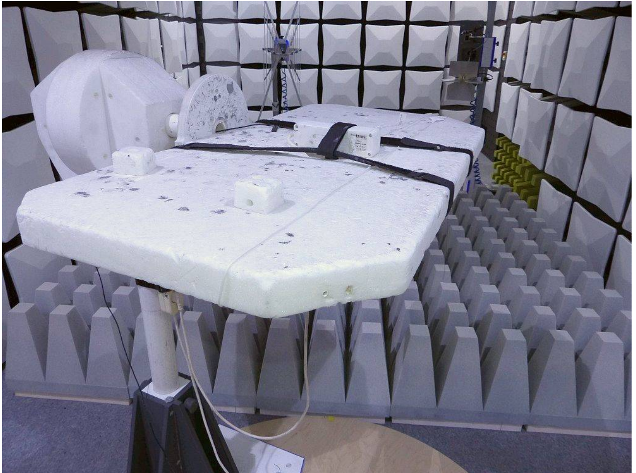
Photo 3: Test setup for radiated measurements (Enclosure, fully-anechoic chamber, 1-26.5 GHz intentional radiator §15, ANSI C63.10 (view from left side))
