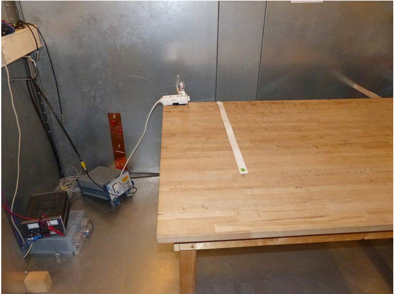
Photo 5: Test setup for conducted measurements (AC Port (power line), EUT supplied by AC/DC adapter, intentional radiator §15, ANSI C63.10)
