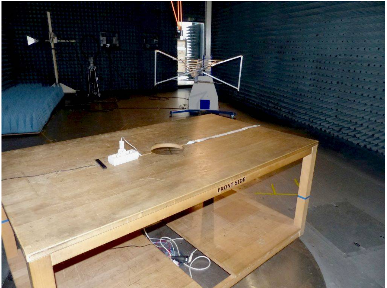
Photo 7: Test setup for radiated measurements (AC Port (power line), EUT supplied by AC/DC adapter, unintentional radiator §15.109, ANSI C63.4)
