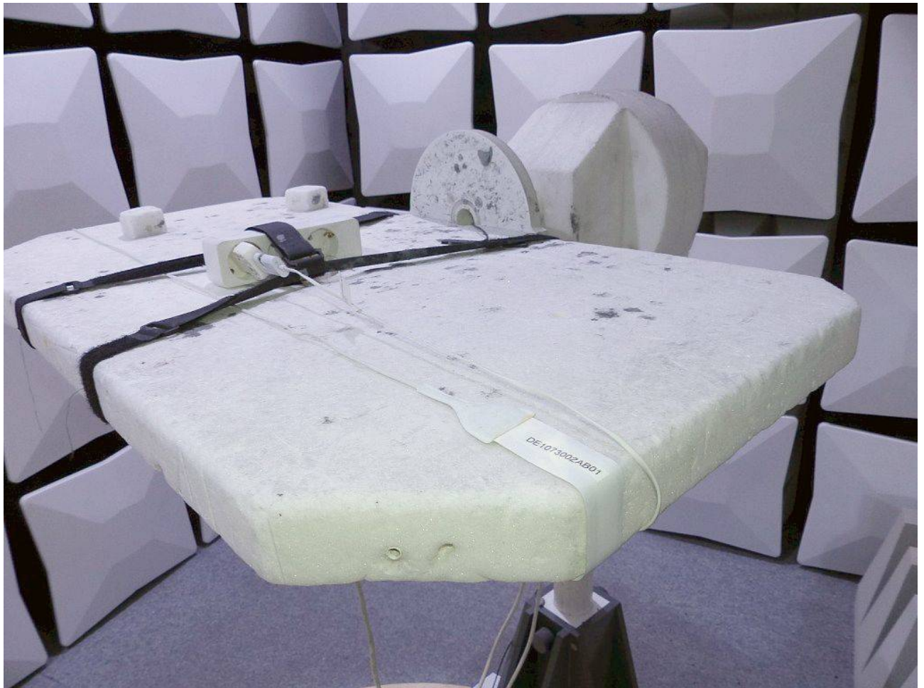
Photo 4: Test setup for radiated measurements (Enclosure, fully-anechoic chamber, 1-26.5 GHz intentional radiator §15, ANSI C63.10 (view from right side)
