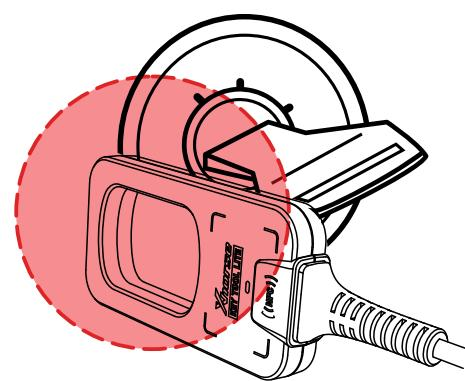
As shown in the figure, move the KEY TOOL LITE close to the ignition switch, and turn the ignition key on and off repeatedly. (For push start system, use the KEY TOOL LITE close to the emergency switch area, then press the start button repeatedly.)
