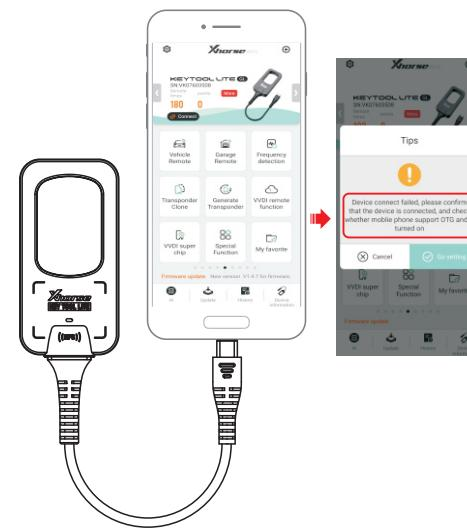
**Power on:** Insert the TYPE-C cable, and allow the app to access the USB port of the phone, and connect the device.
