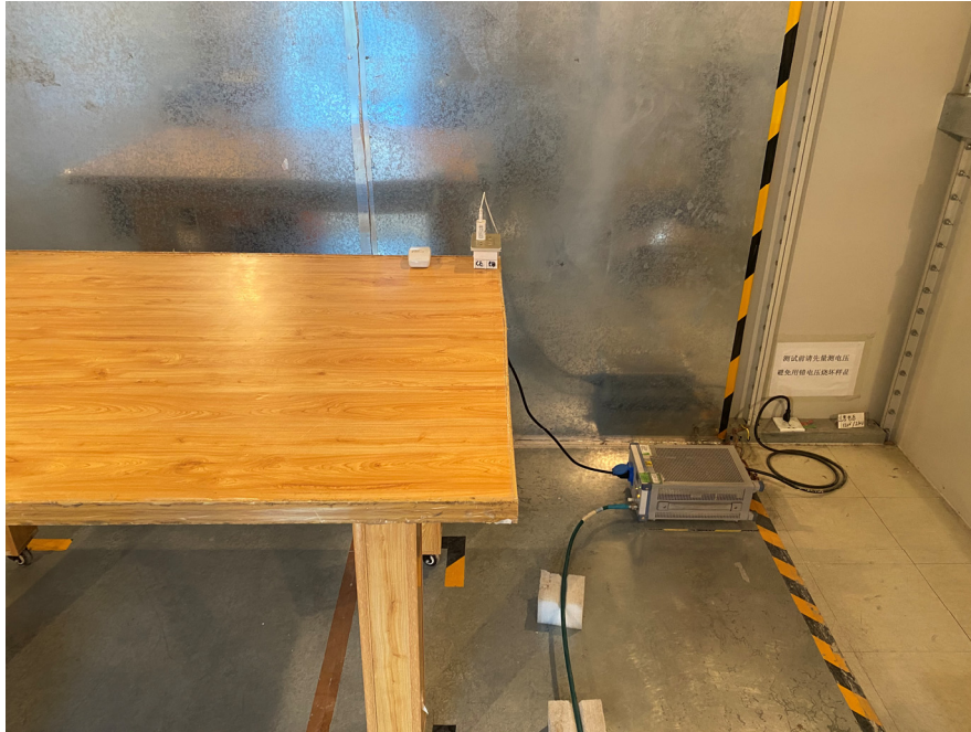
Conducted Emissions (Side View)
