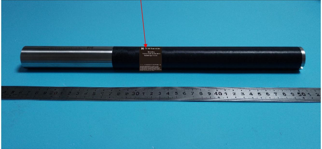
The label shown shall be permanently affixed at a conspicuous location on the device and be readily visible to the user at the time purchase (Labeling requirements per 2.925)
