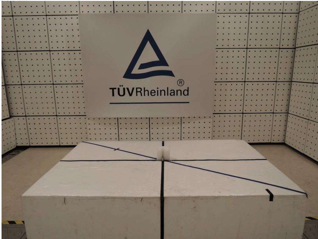
Photograph 1: Set-up for Spurious Emissions (Front View)
