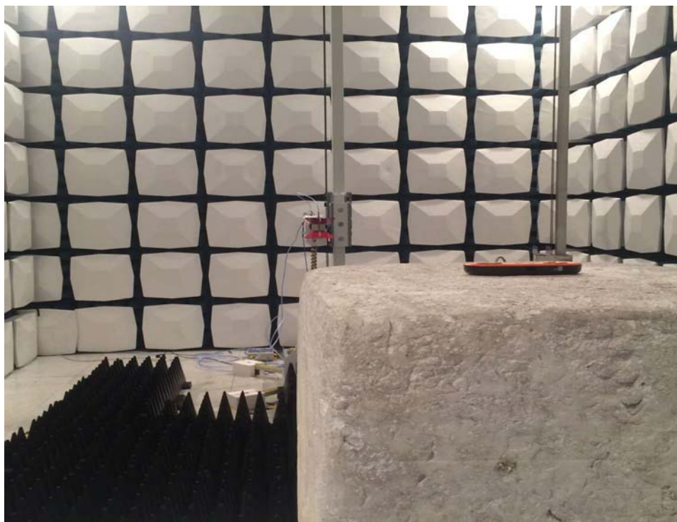
Description: Radiated Emission Test Setup for 1~18GHz
