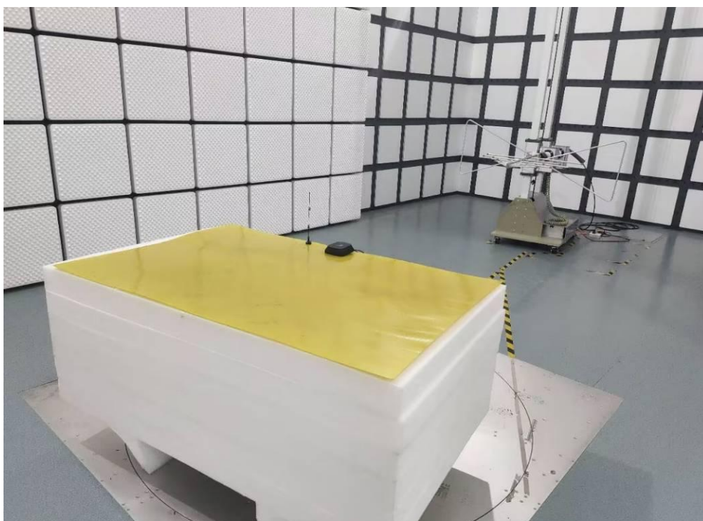
Photo of Radiated Emission Measurement (Below 1G)
