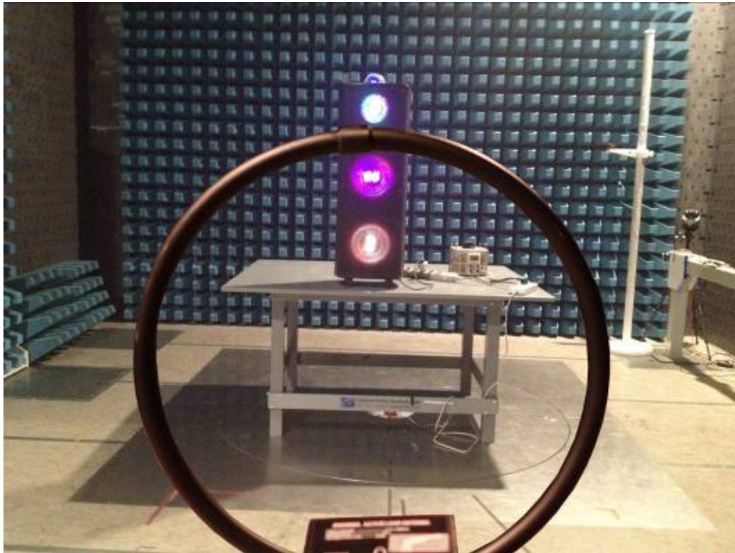
Re, Tested by Active Loop Antenna
