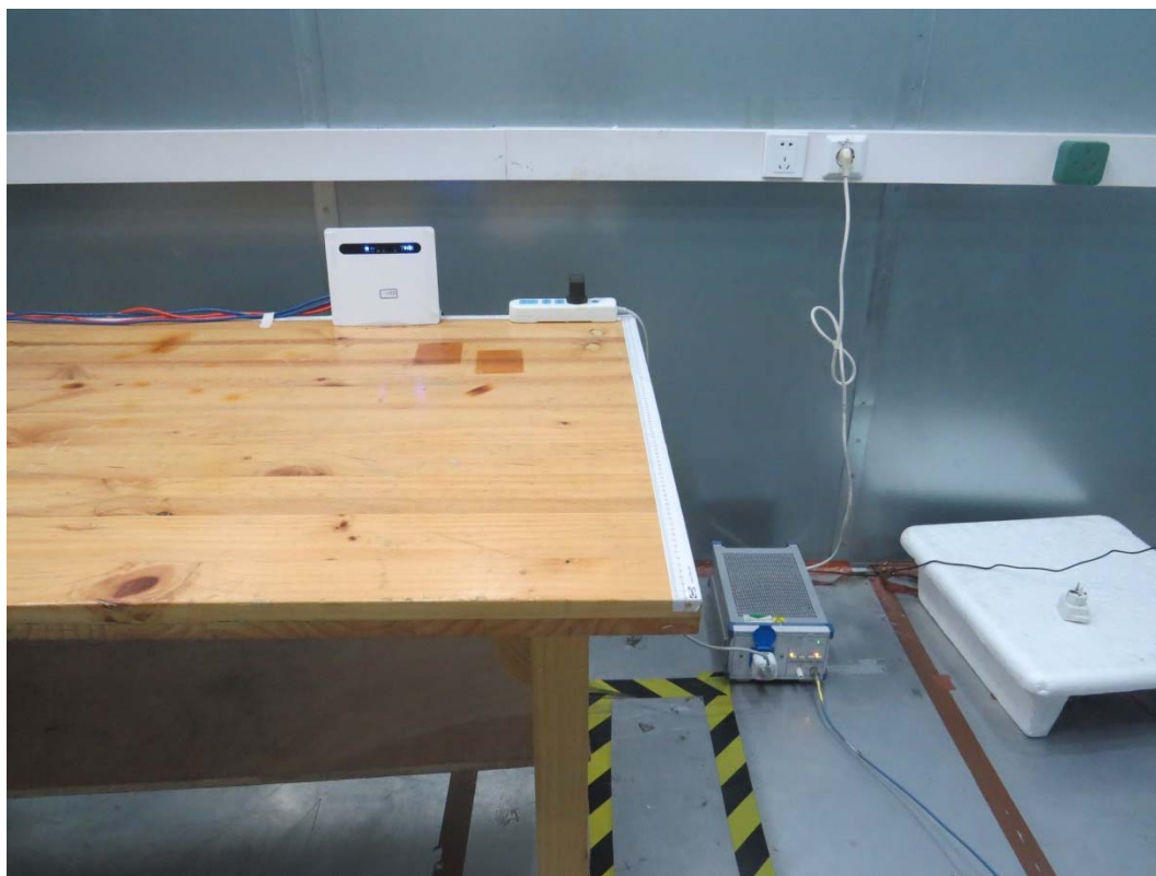
Picture 3 Conducted Emission Test Setup
