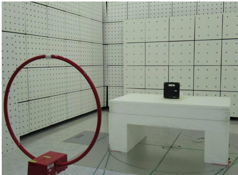
**Radiated Emission Set up Photos (Below 1GHz)**
