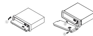
Before detaching the front panel. Make sure to power off the unit. Press ① to loosen the panel and slide it to the right side to release the panel and then pull it off towards you.
