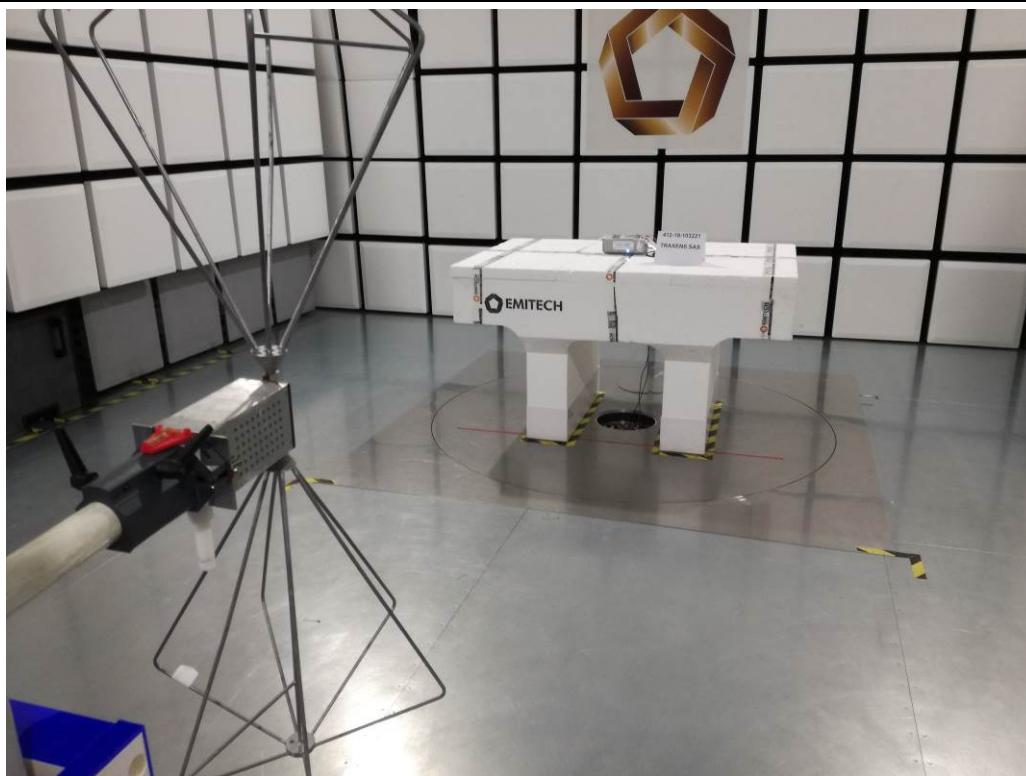
TEST SETUP PHOTO(S) – FREQ < 200MHz
