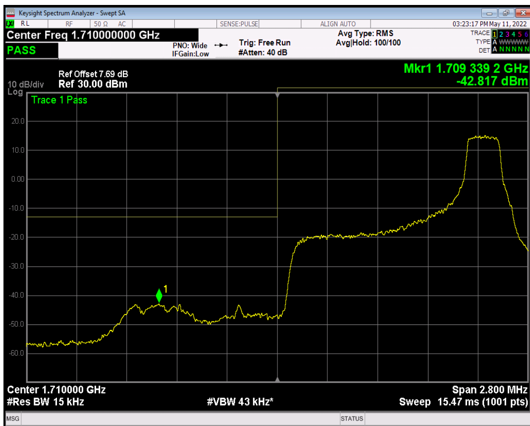
Band66 QPSK BW=1.4MHz Channel=131979 RB Size=6 Position=#0
