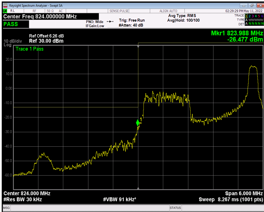
Band5 QAM16 BW=3MHz Channel=20415 RB Size=15 Position=#0
