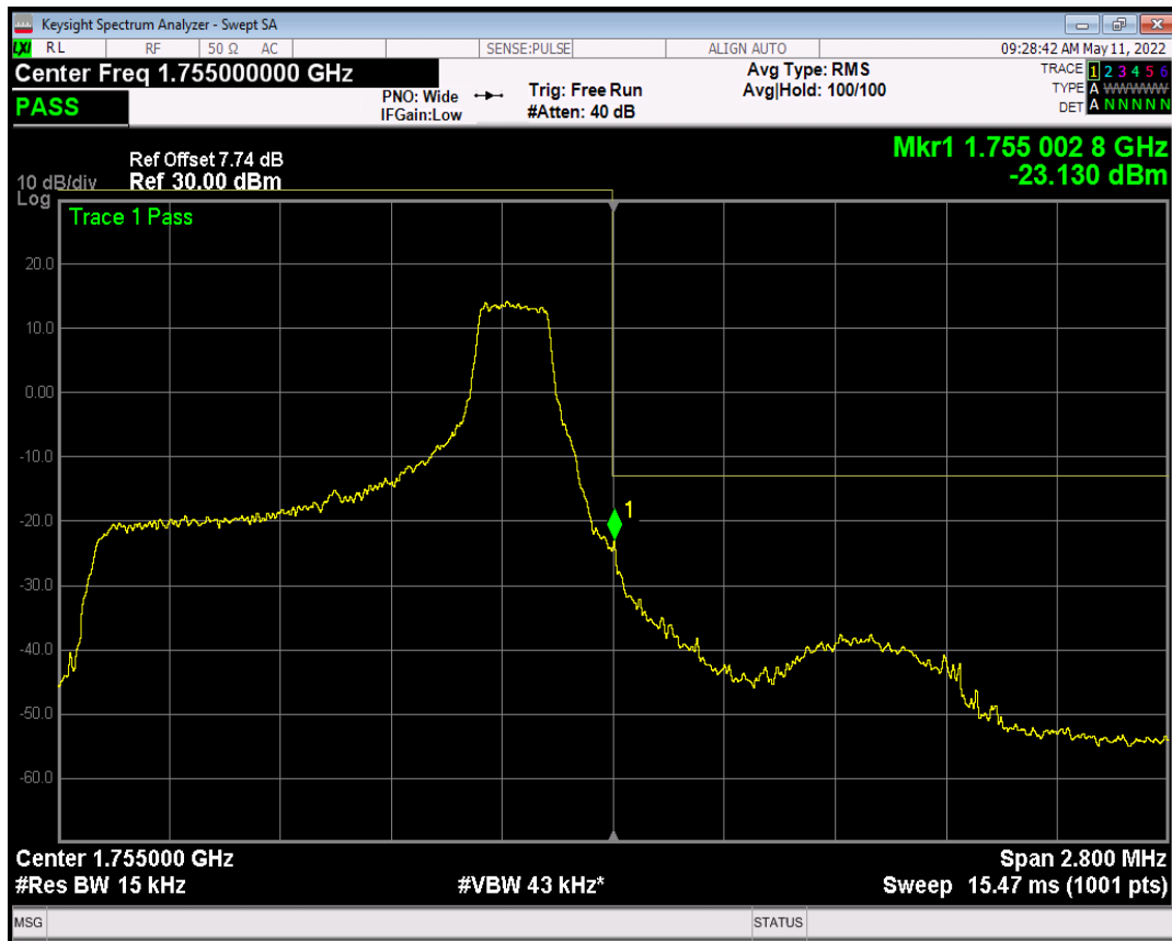
Band4 QAM16 BW=1.4MHz Channel=20393 RB Size=6 Position=#0
