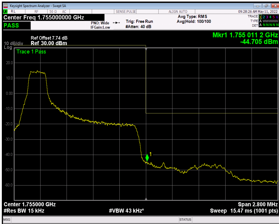
Band4 QPSK BW=1.4MHz Channel=20393 RB Size=1 Position=#Max
