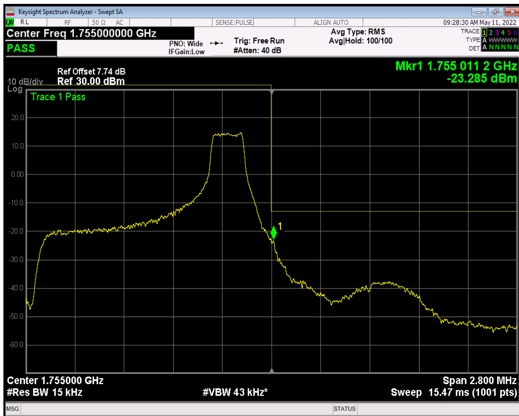
Band4 QPSK BW=1.4MHz Channel=20393 RB Size=6 Position=#0
