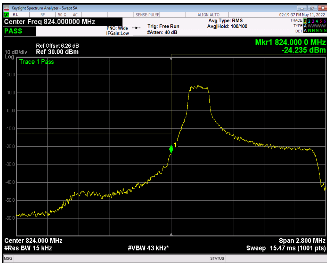
Band5 QPSK BW=1.4MHz Channel=20407 RB Size=1 Position=#Max
