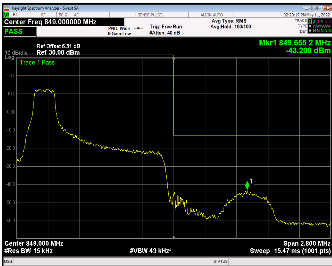
Band5 QAM16 BW=1.4MHz Channel=20643 RB Size=1 Position=#Max
