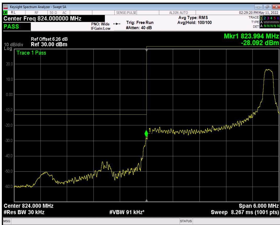
Band5 QPSK BW=3MHz Channel=20415 RB Size=15 Position=#0
