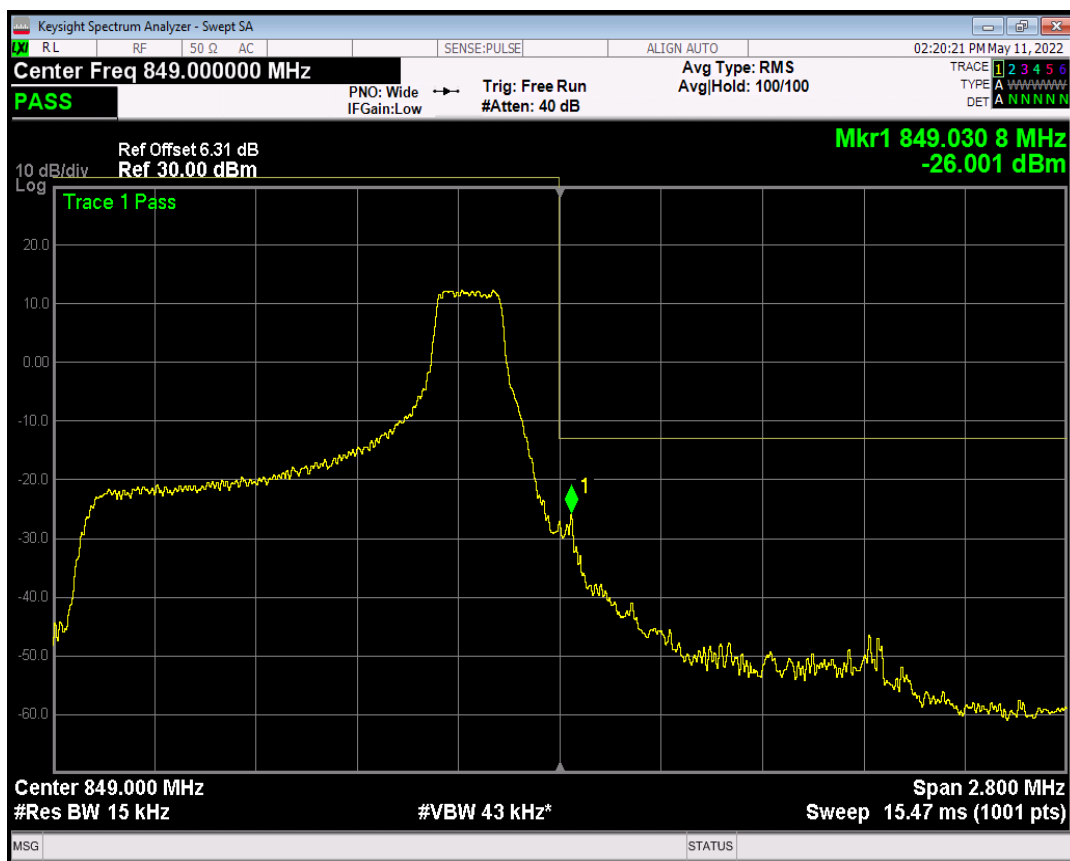
Band5 QAM16 BW=1.4MHz Channel=20643 RB Size=6 Position=#0
