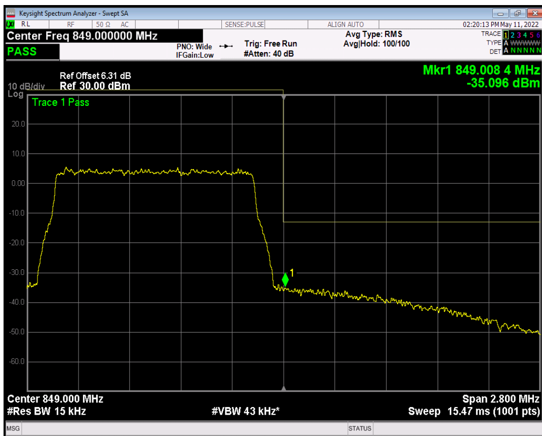
Band5 QAM16 BW=1.4MHz Channel=20643 RB Size=1 Position=#0
