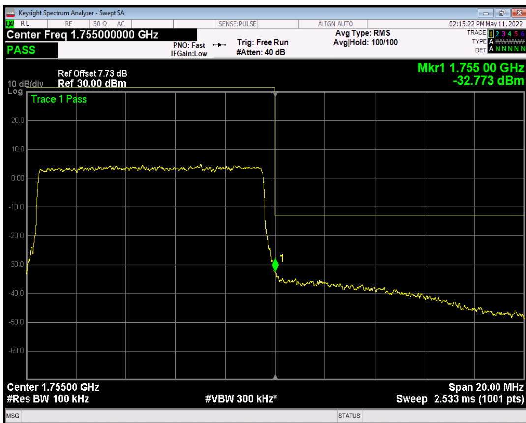
Band4 QPSK BW=15MHz Channel=20025 RB Size=1 Position=#0
