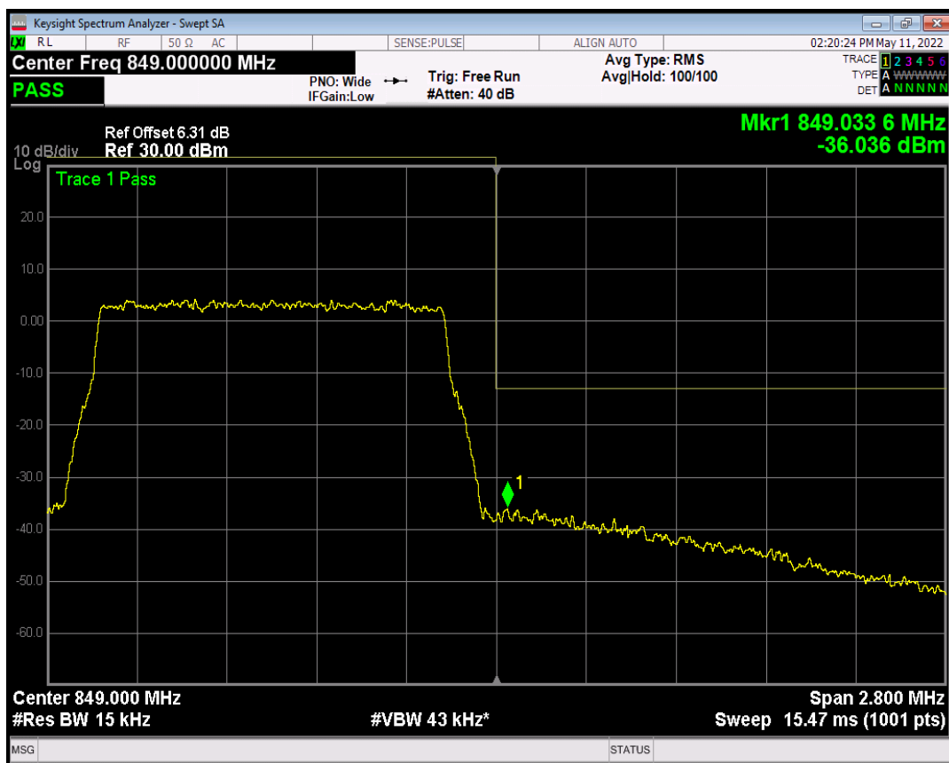
Band5 QPSK BW=3MHz Channel=20415 RB Size=1 Position=#0
