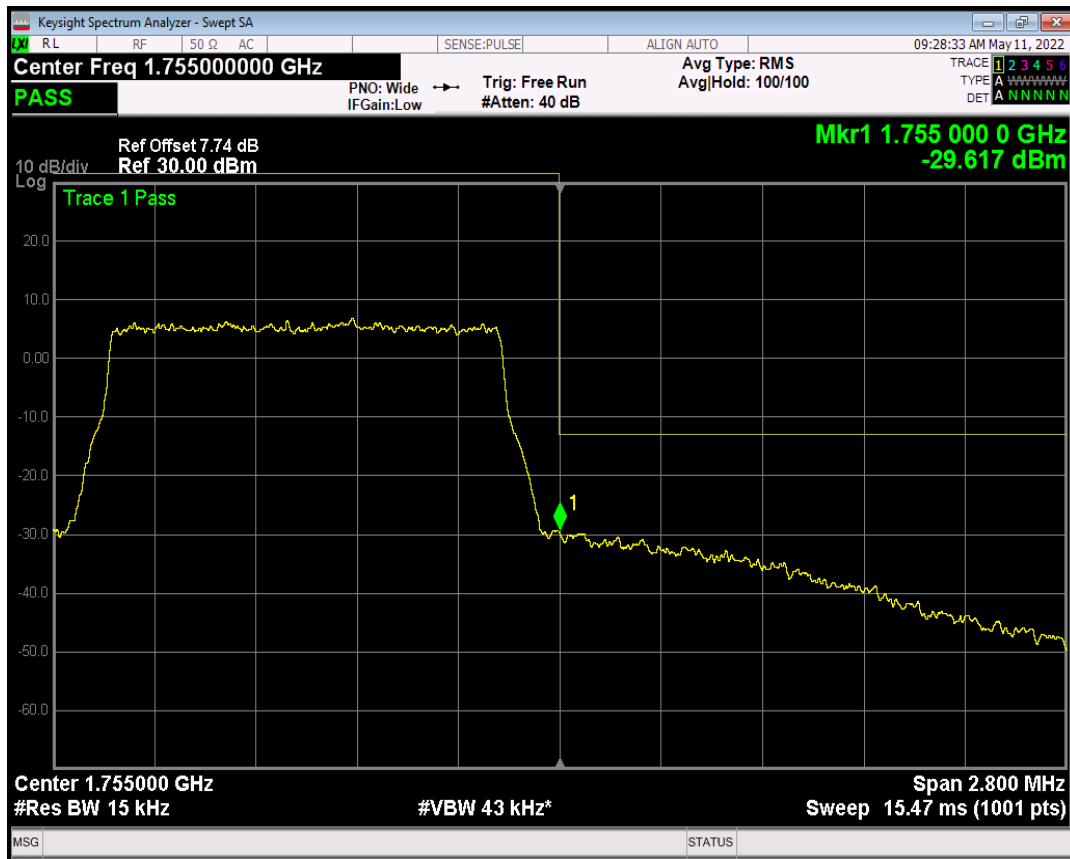
Band4 QAM16 BW=1.4MHz Channel=20393 RB Size=1 Position=#0
