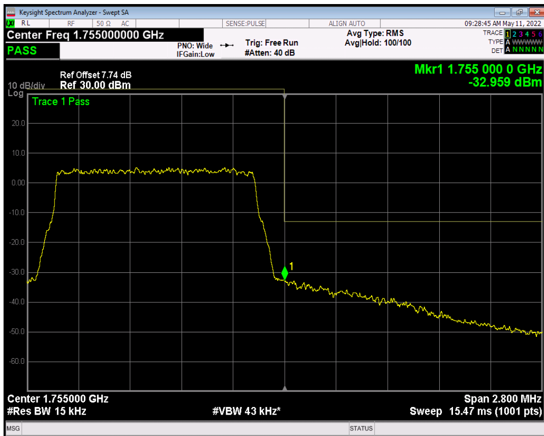
Band4 QPSK BW=5MHz Channel=19975 RB Size=1 Position=#0
