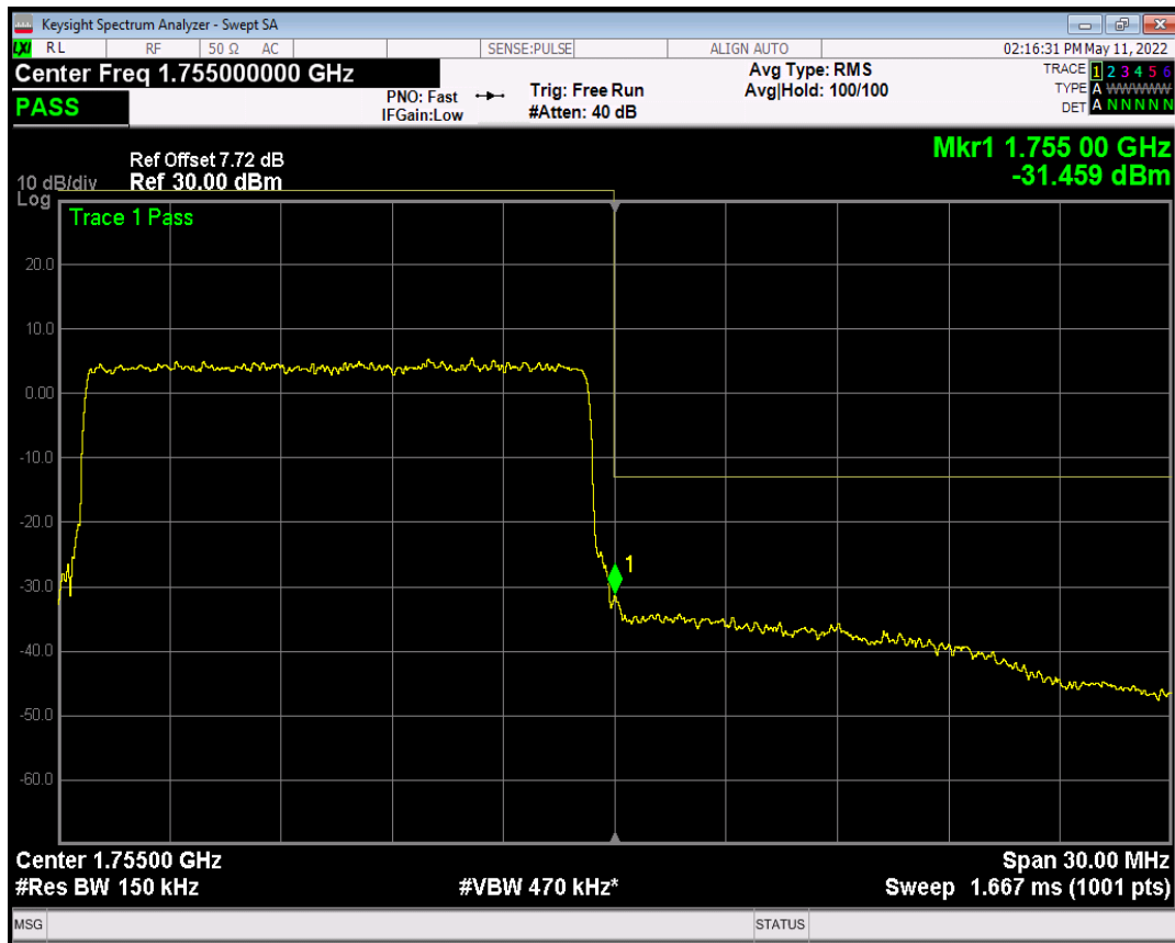
Band4 QAM16 BW=15MHz Channel=20325 RB Size=1 Position=#0
