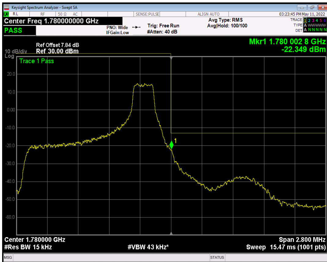
Band66 QPSK BW=1.4MHz Channel=132665 RB Size=6 Position=#0
