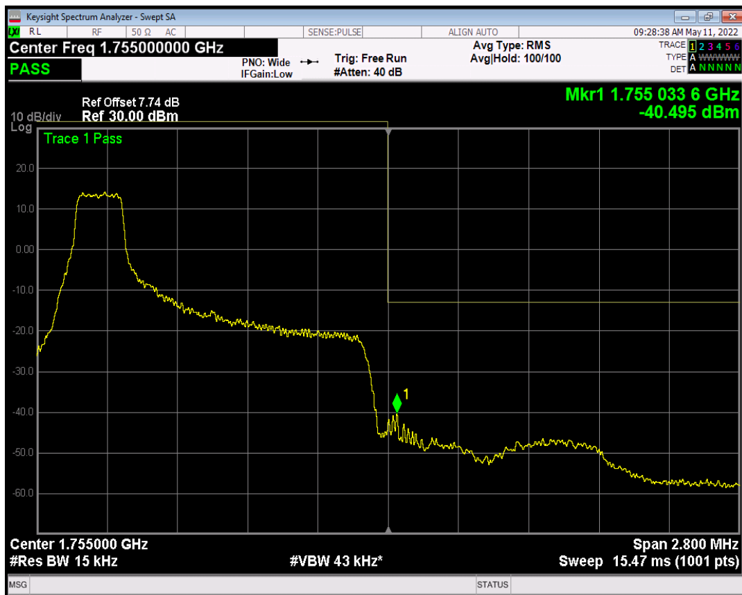
Band4 QAM16 BW=1.4MHz Channel=20393 RB Size=1 Position=#Max
