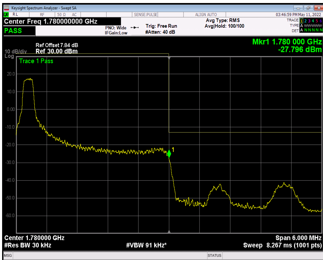
Band66 QPSK BW=3MHz Channel=132657 RB Size=1 Position=#Max
