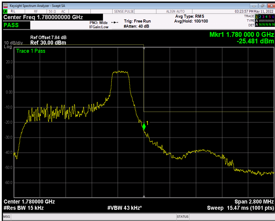
Band66 QAM16 BW=1.4MHz Channel=132665 RB Size=6 Position=#0
