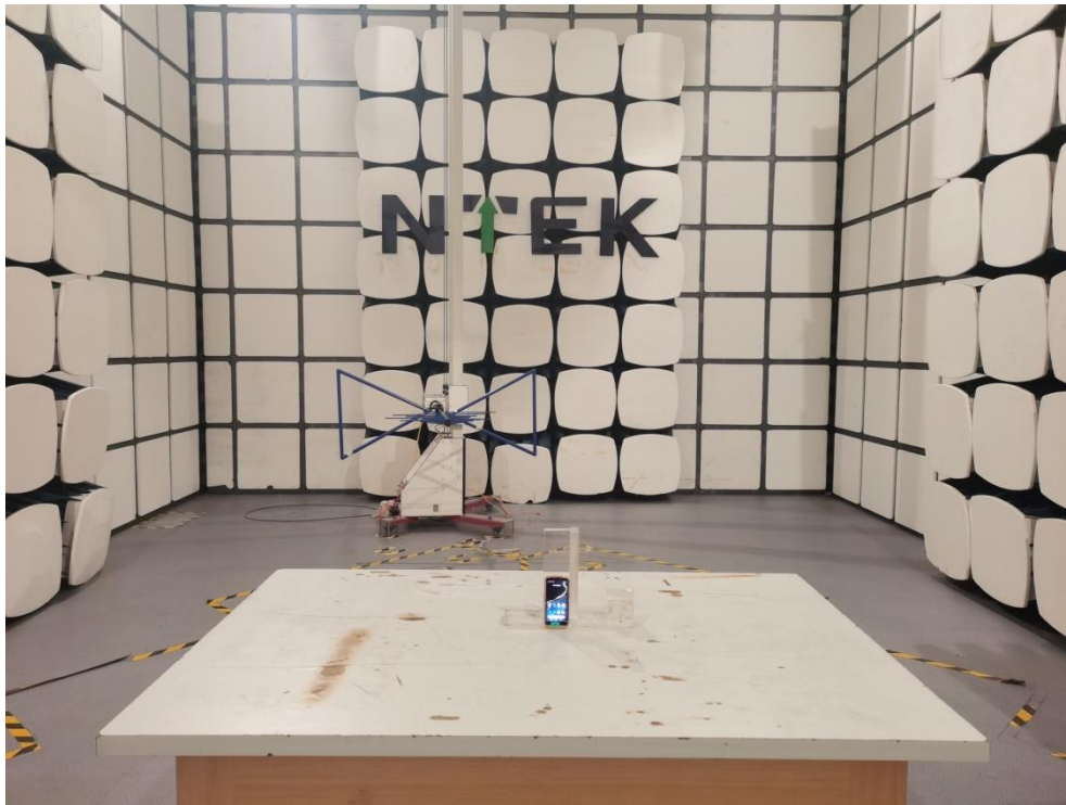
Radiated Measurement Photos(30MHz~1GHz )
