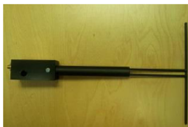
Figure 1 – MVG COMOSAR Validation Dipole
