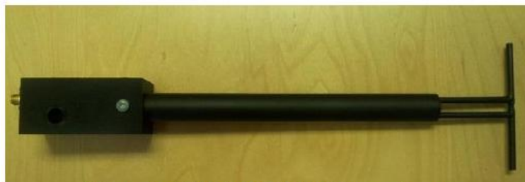
Figure 1 – MVG COMOSAR Validation Dipole
