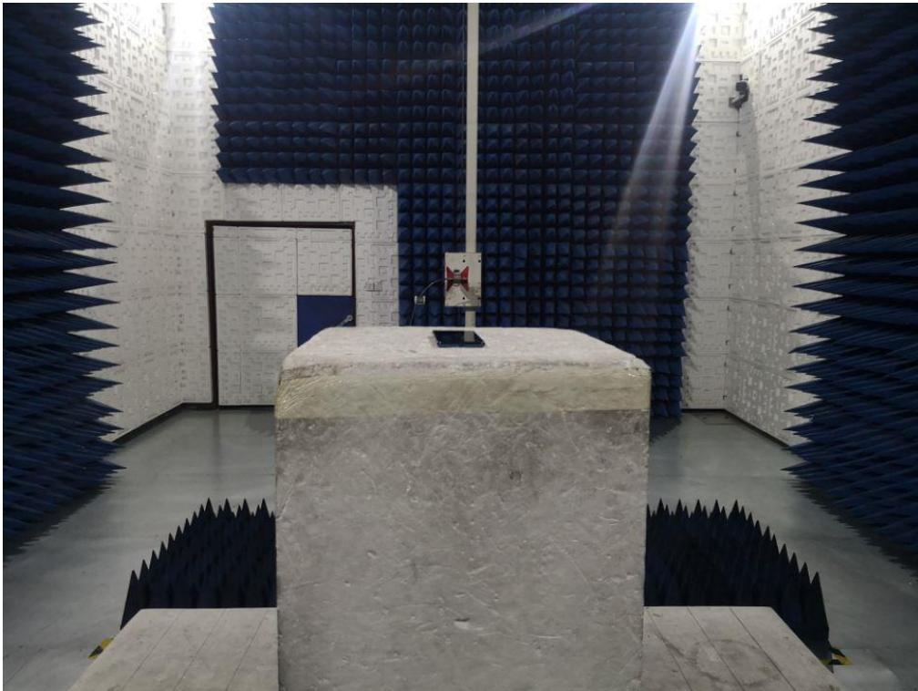
RADIATED EMISSION TEST SETUP ABOVE 1GHz
