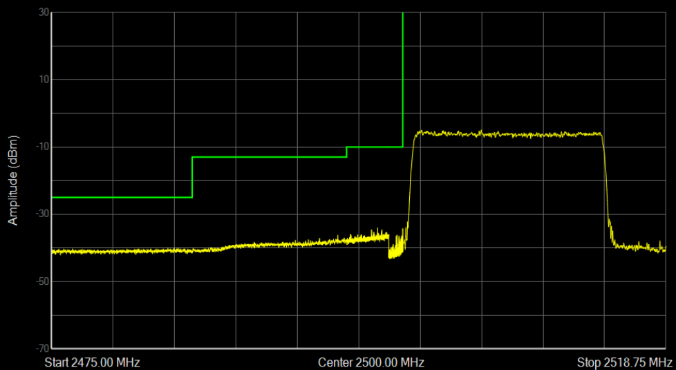
Band7 QPSK BW=15MHz Channel=20825 RB Size=75 Position=#0
