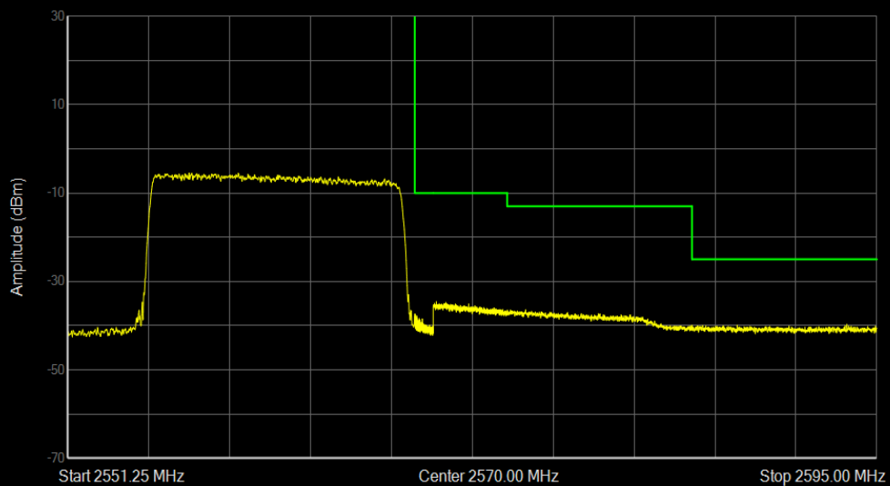
Band7 QPSK BW=15MHz Channel=21375 RB Size=75 Position=#0
