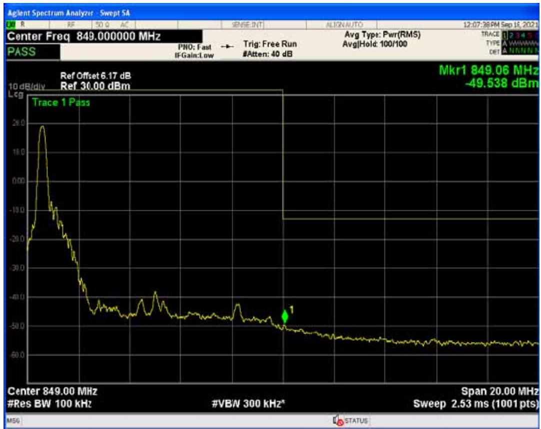
Band5 QAM16 BW=10MHz Channel=20600 RB Size=1 Position=#Max
