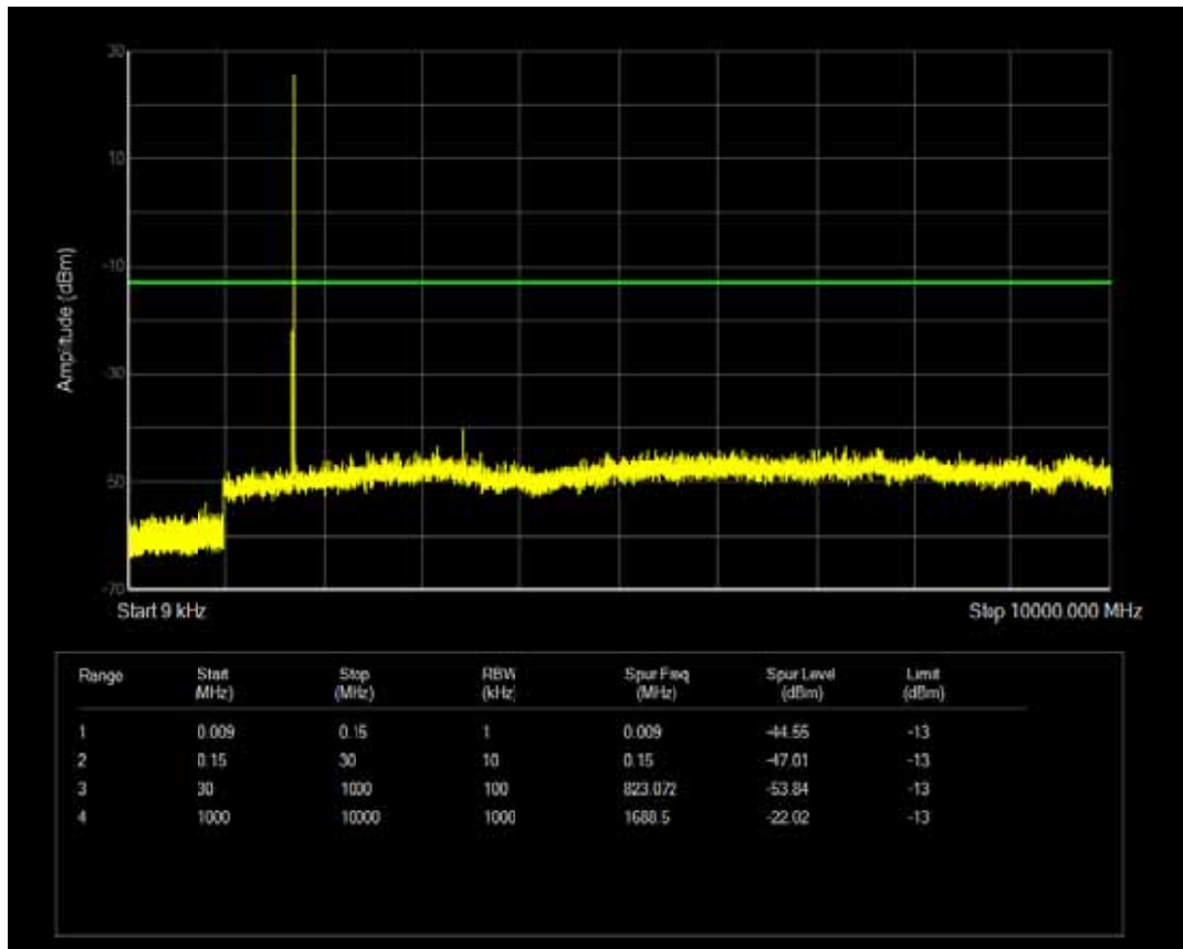
Band4 QPSK BW=1.4MHz Channel=19957 RB Size=1 Position=#0
