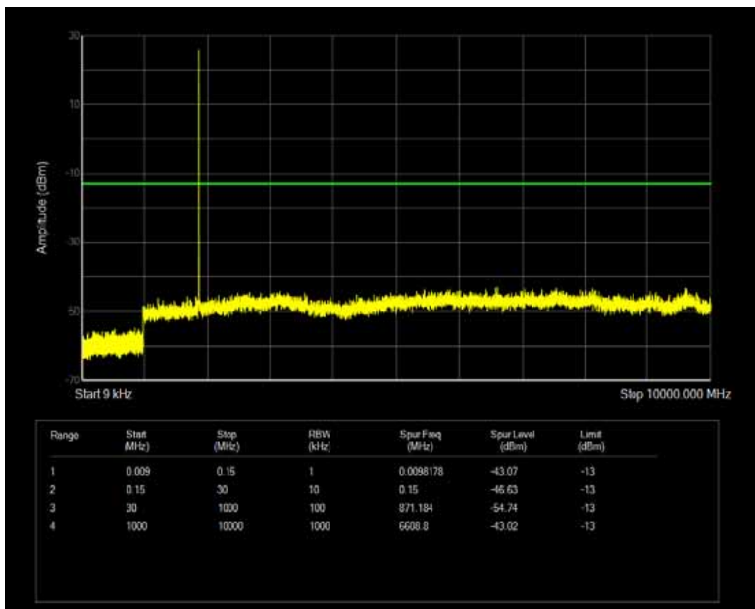
Band2 QPSK BW=1.4MHz Channel=19193 RB Size=1 Position=#0
