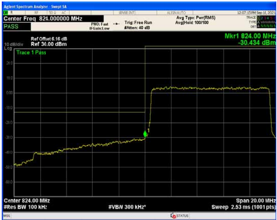
Band5 QPSK BW=10MHz Channel=20450 RB Size=1 Position=#Max
