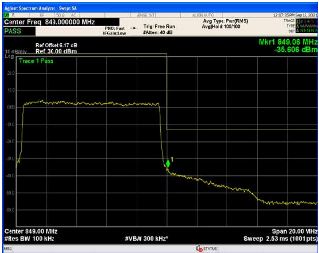
Band5 QAM16 BW=10MHz Channel=20600 RB Size=1 Position=#0
