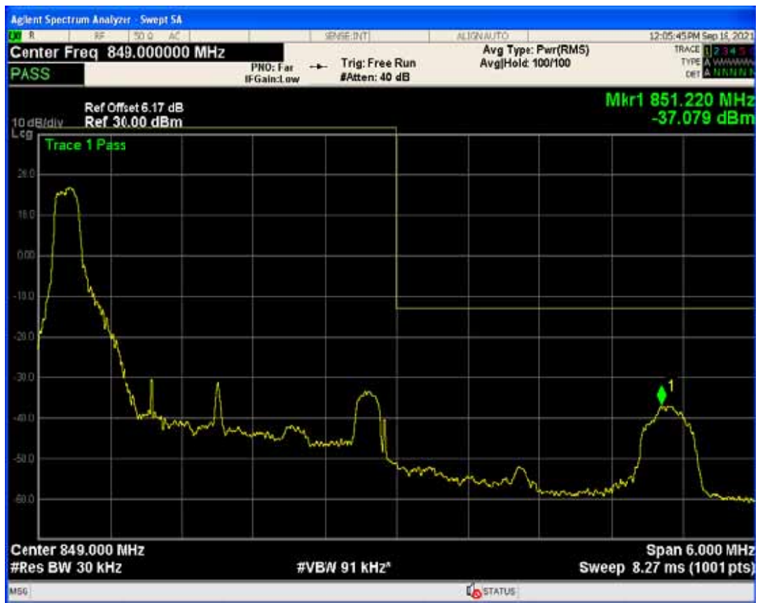
Band5 QAM16 BW=3MHz Channel=20415 RB Size=15 Position=#0
