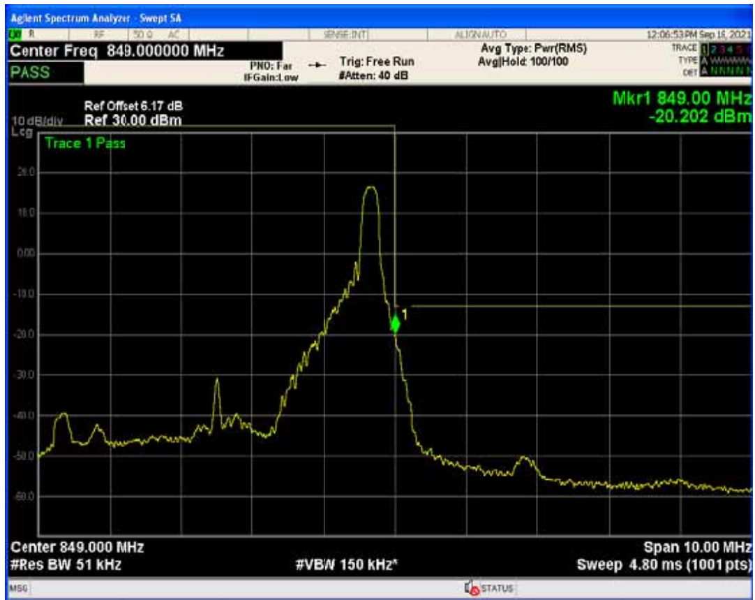
Band5 QPSK BW=10MHz Channel=20450 RB Size=1 Position=#0
