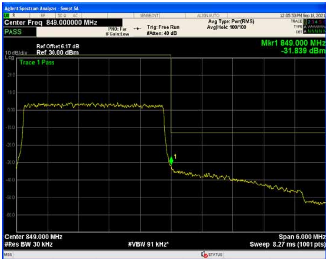
Band5 QAM16 BW=3MHz Channel=20635 RB Size=1 Position=#0
