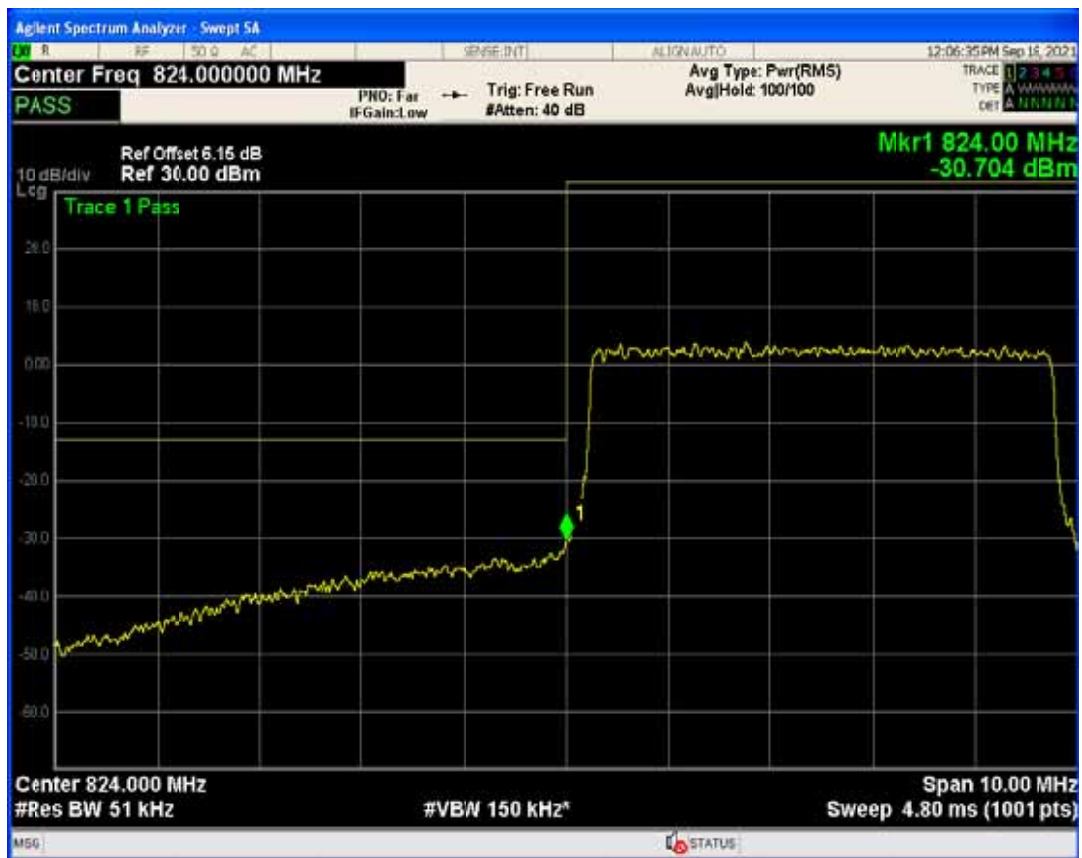
Band5 QAM16 BW=5MHz Channel=20425 RB Size=1 Position=#Max
