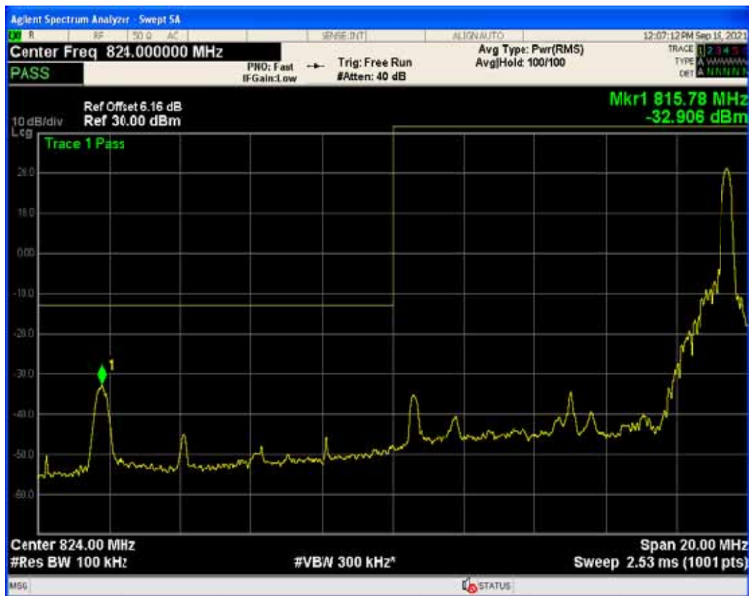
Band5 QAM16 BW=10MHz Channel=20450 RB Size=1 Position=#0
