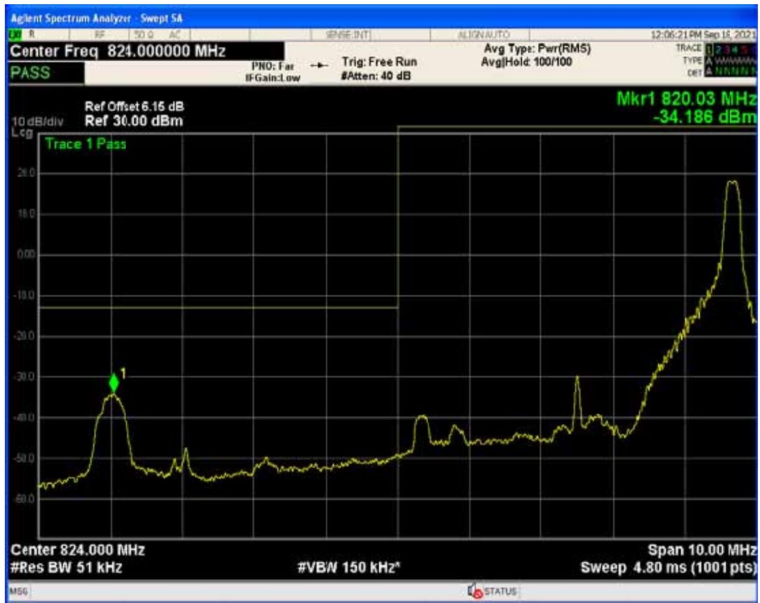
Band5 QPSK BW=5MHz Channel=20425 RB Size=25 Position=#0
