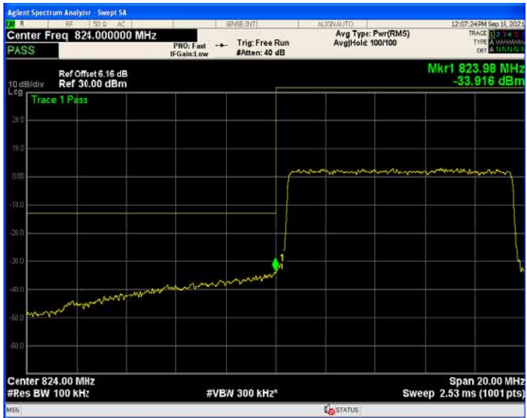
Band5 QPSK BW=10MHz Channel=20600 RB Size=1 Position=#0
