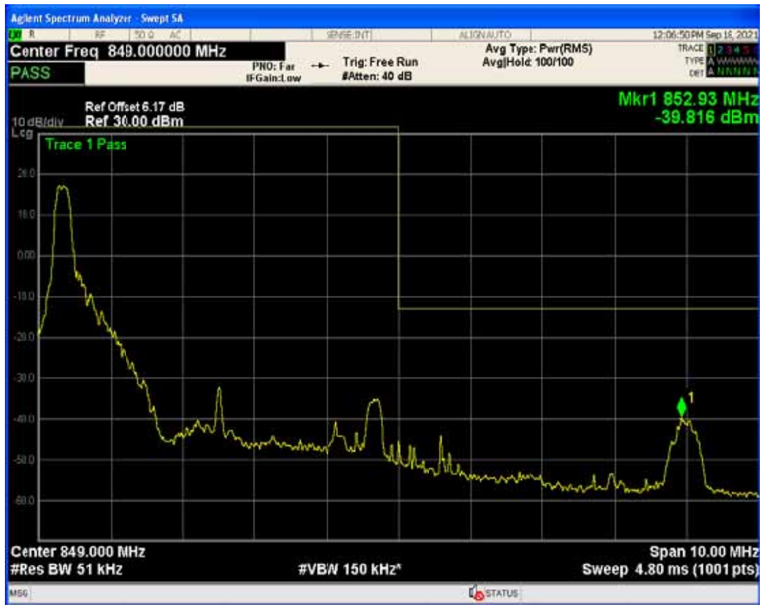
Band5 QAM16 BW=5MHz Channel=20625 RB Size=25 Position=#0
