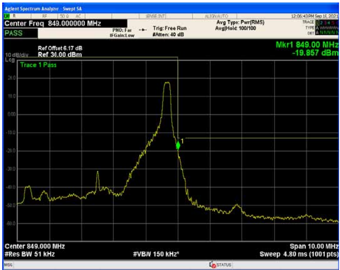
Band5 QPSK BW=5MHz Channel=20625 RB Size=25 Position=#0
