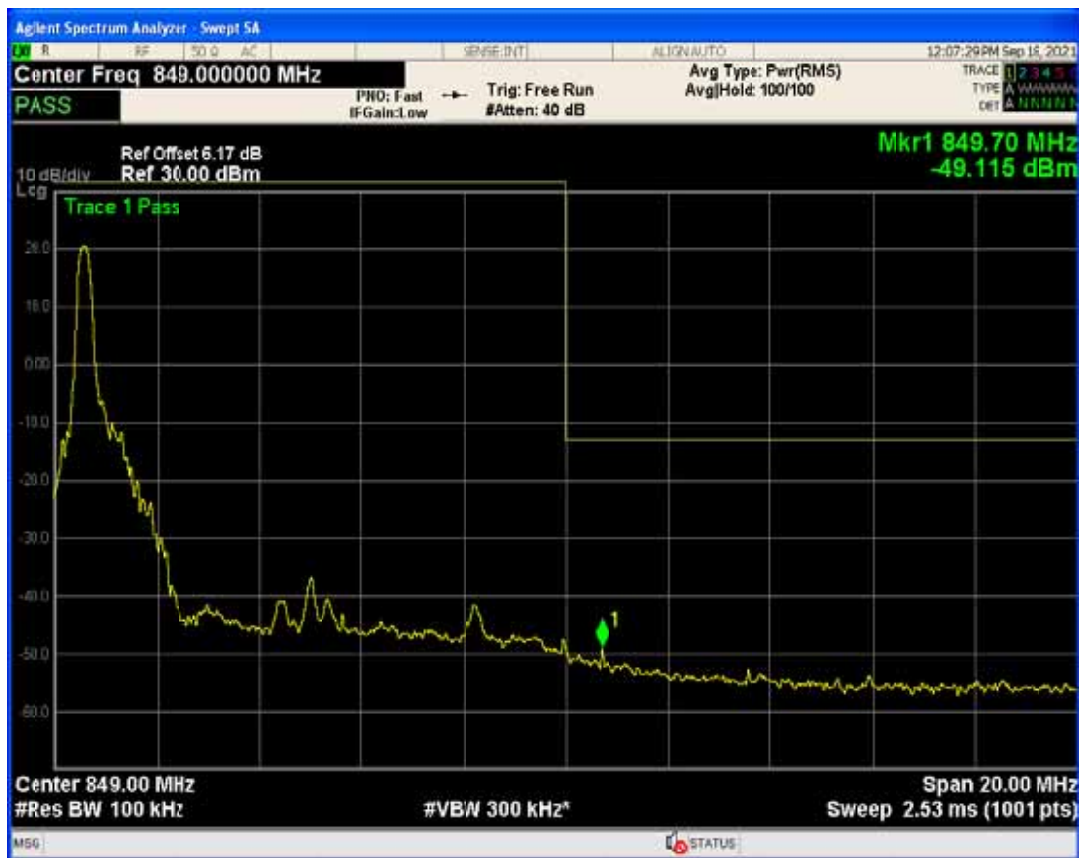
Band5 QPSK BW=10MHz Channel=20600 RB Size=1 Position=#Max
