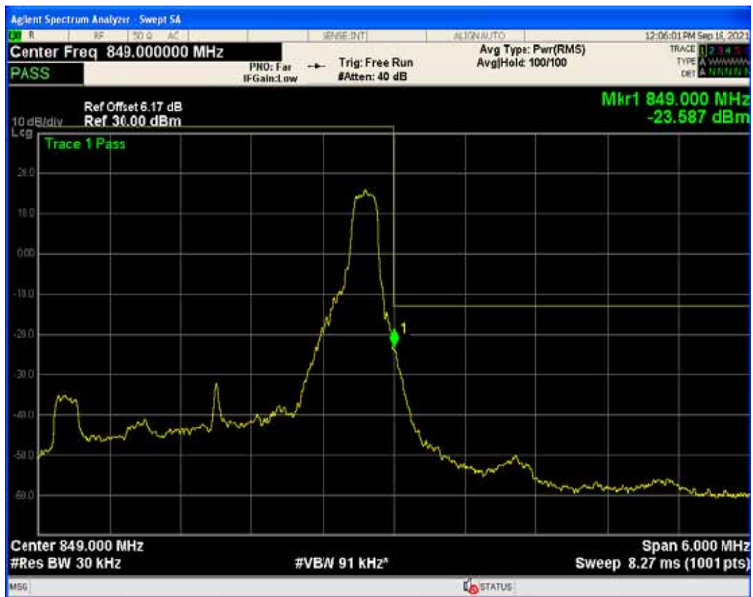
Band5 QPSK BW=5MHz Channel=20425 RB Size=1 Position=#0
