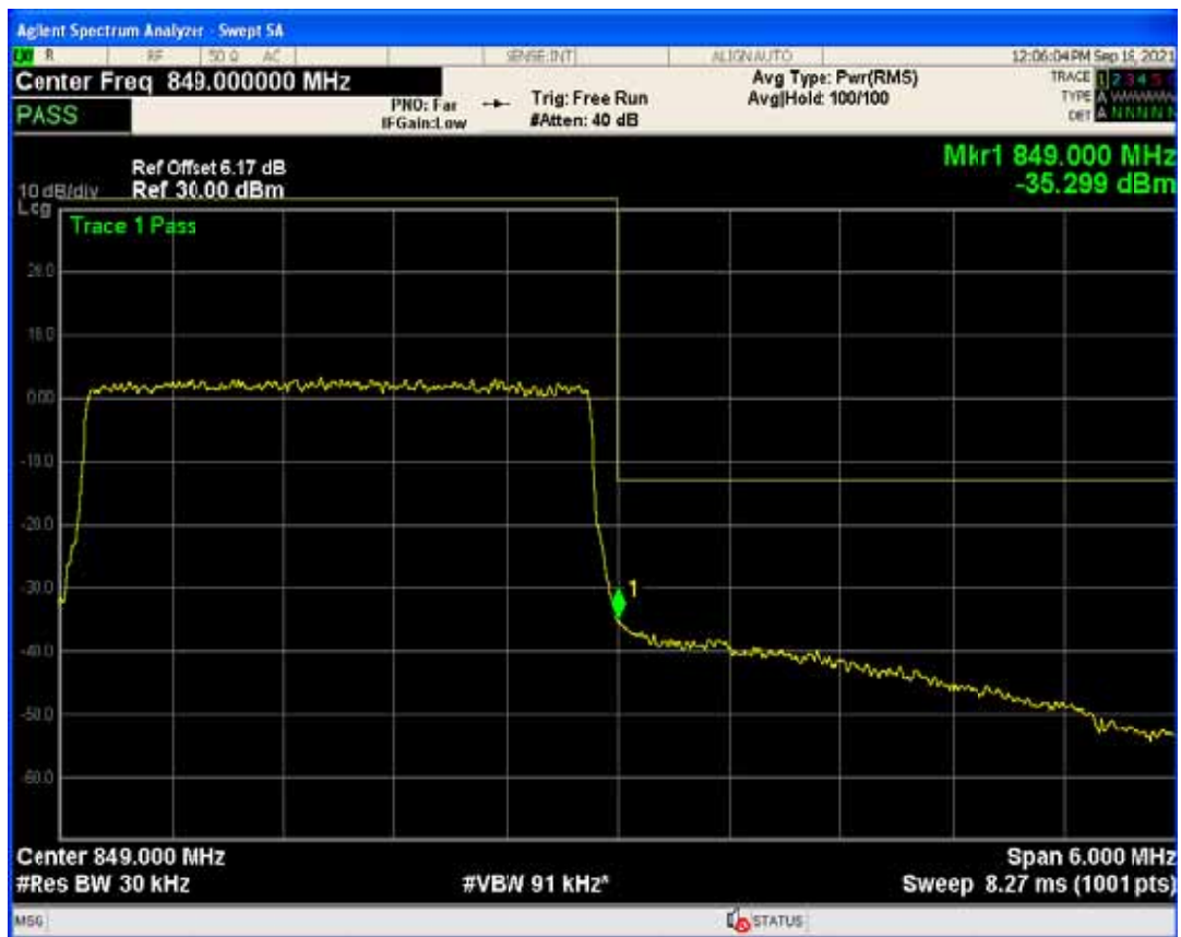
Band5 QPSK BW=5MHz Channel=20425 RB Size=1 Position=#Max
