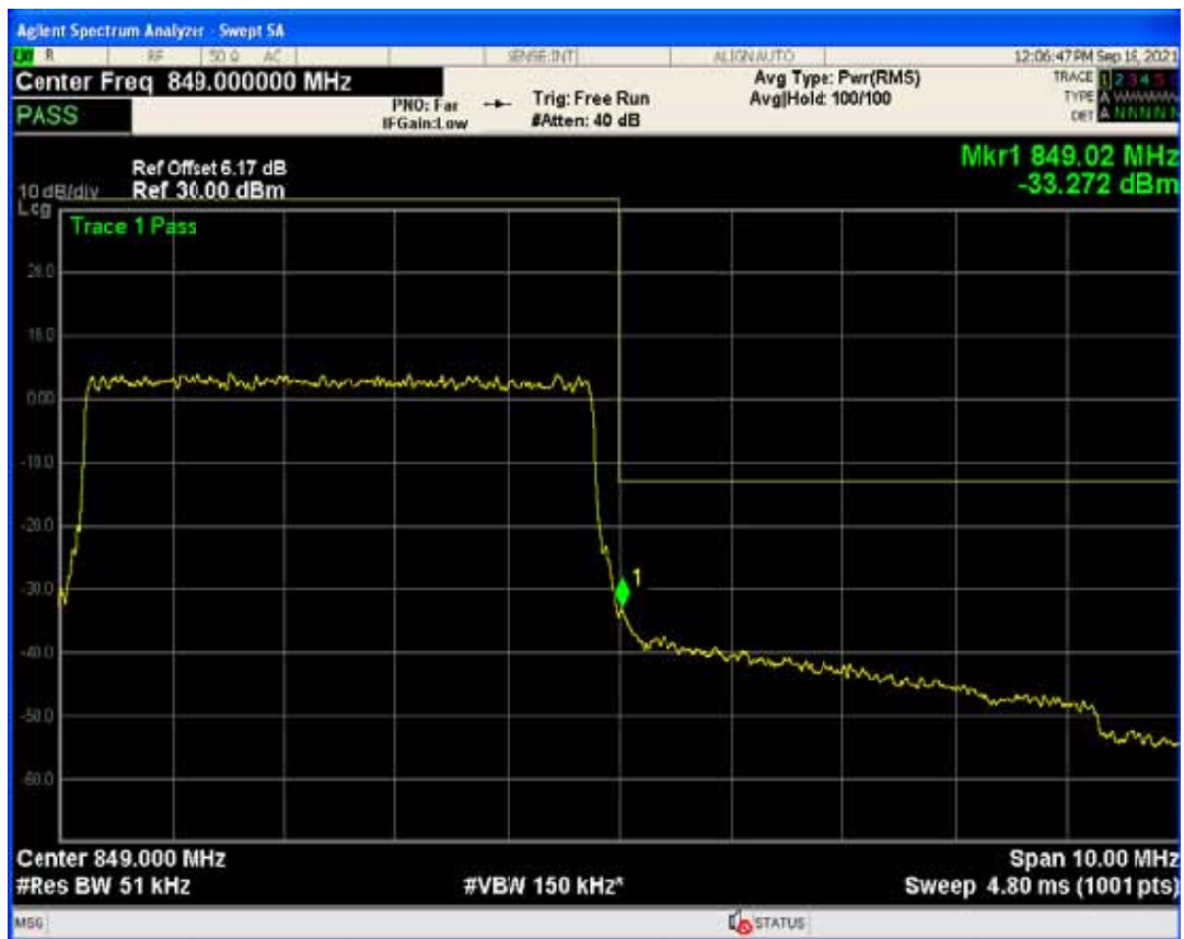
Band5 QAM16 BW=5MHz Channel=20625 RB Size=1 Position=#0
