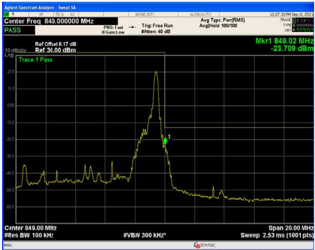
Band5 QPSK BW=10MHz Channel=20600 RB Size=50 Position=#0
