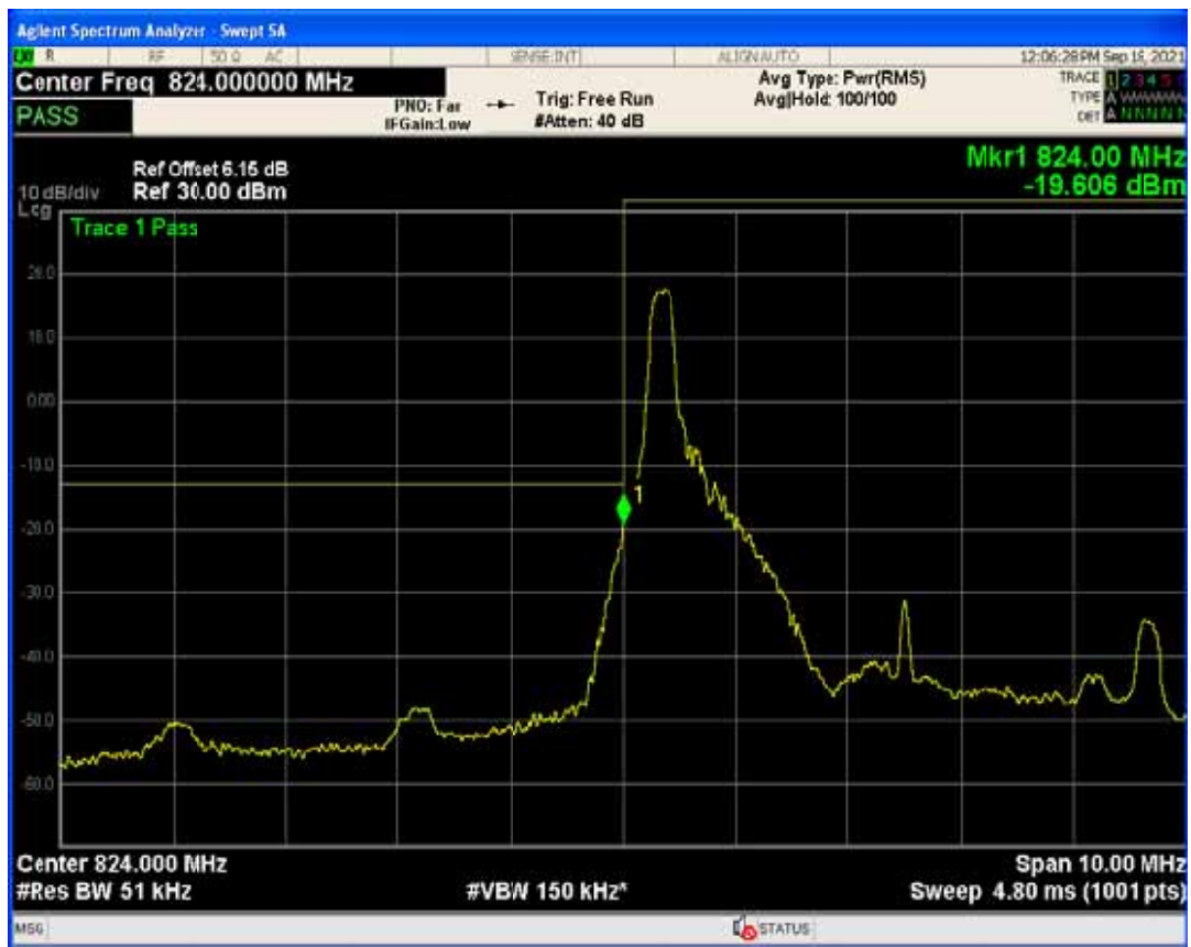
Band5 QAM16 BW=5MHz Channel=20425 RB Size=25 Position=#0
