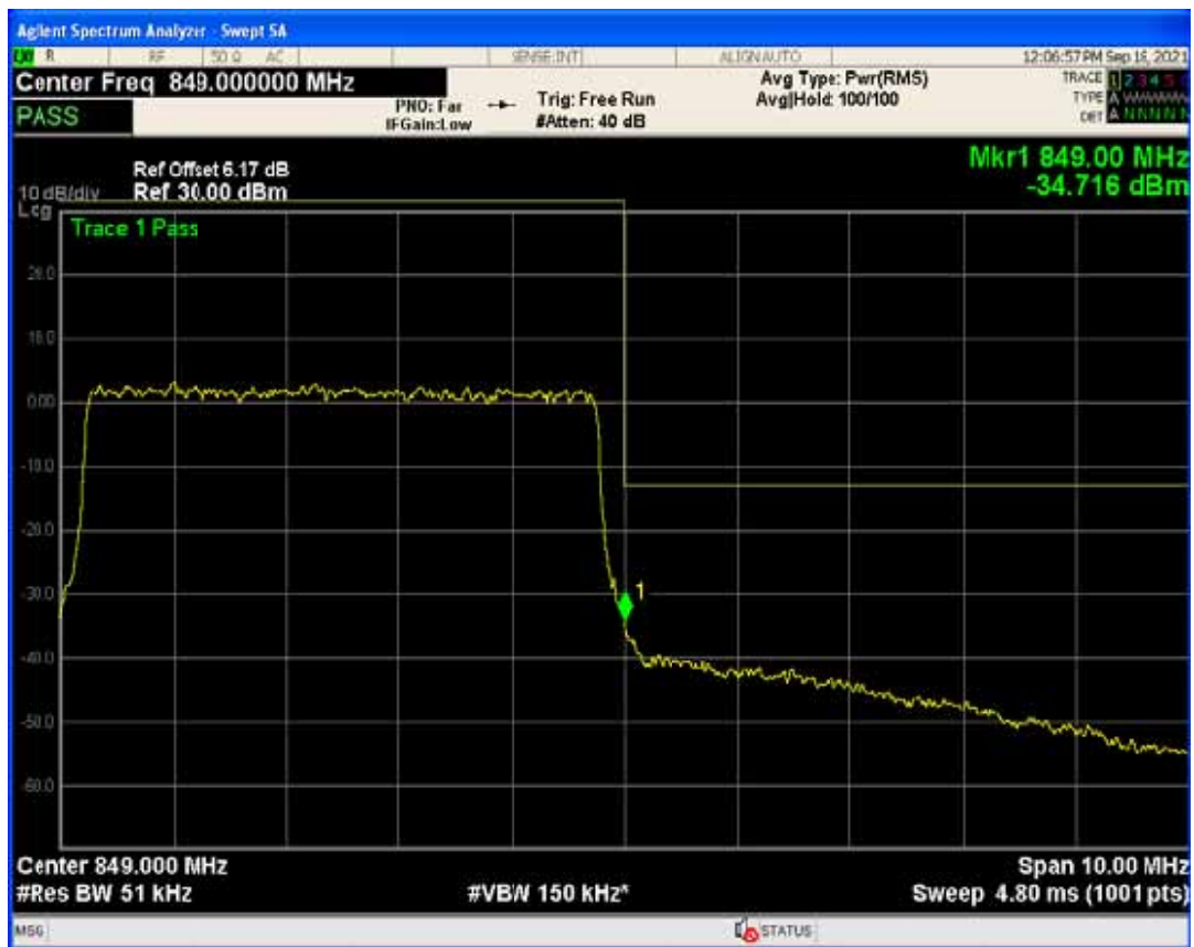
Band5 QAM16 BW=5MHz Channel=20625 RB Size=1 Position=#Max
