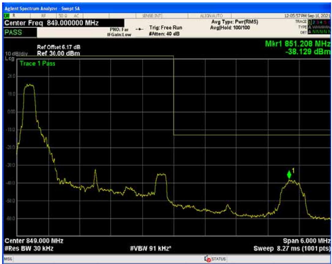
Band5 QAM16 BW=3MHz Channel=20635 RB Size=1 Position=#Max
