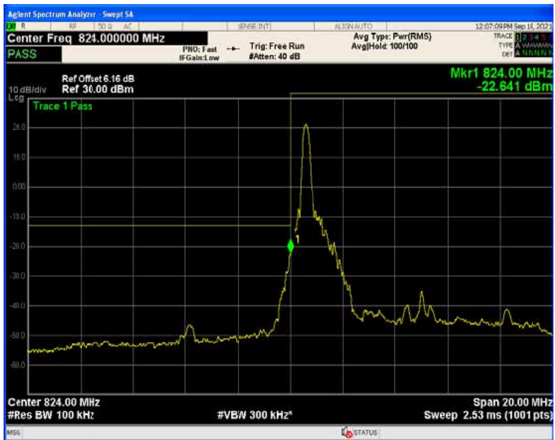
Band5 QPSK BW=10MHz Channel=20450 RB Size=50 Position=#0
