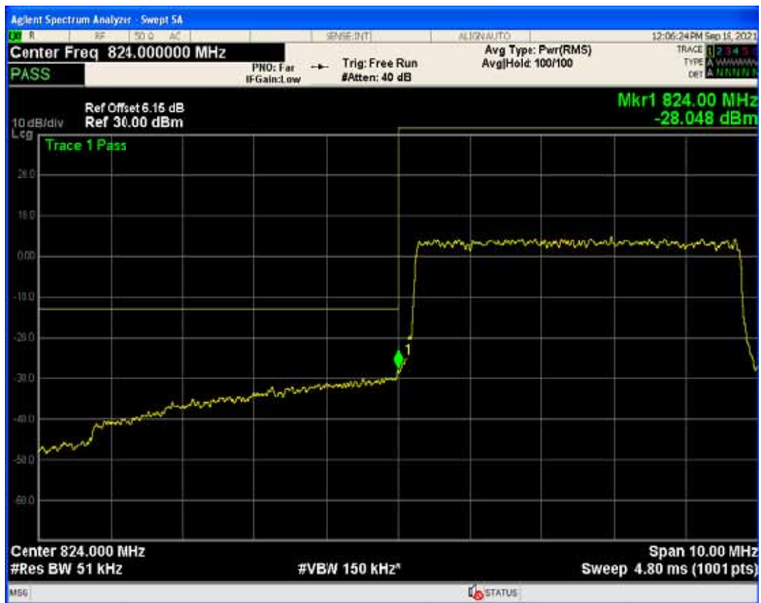
Band5 QAM16 BW=5MHz Channel=20425 RB Size=1 Position=#0
