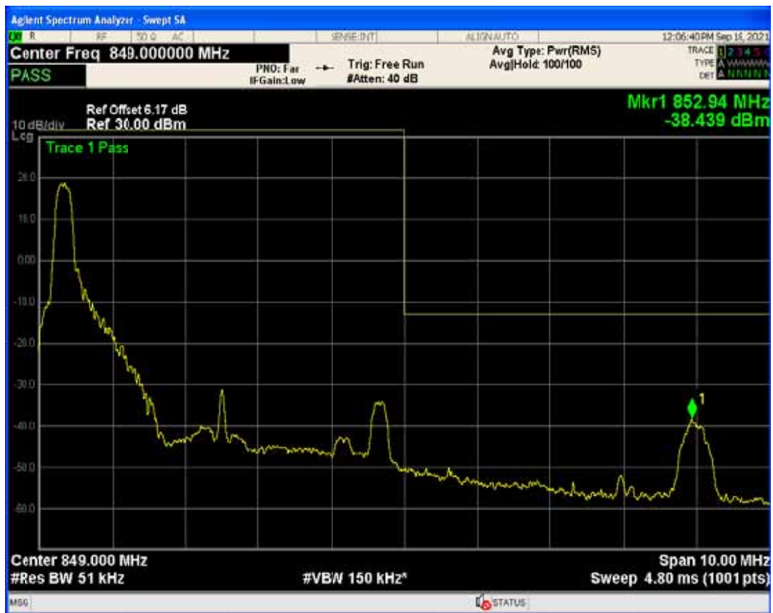
Band5 QPSK BW=5MHz Channel=20625 RB Size=1 Position=#Max
