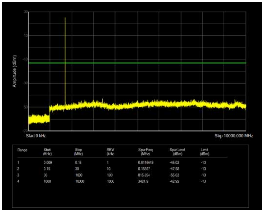
Band4 QPSK BW=1.4MHz Channel=20175 RB Size=1 Position=#0
