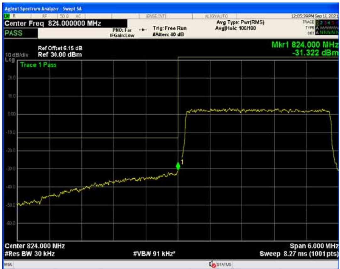
Band5 QPSK BW=3MHz Channel=20635 RB Size=1 Position=#Max
