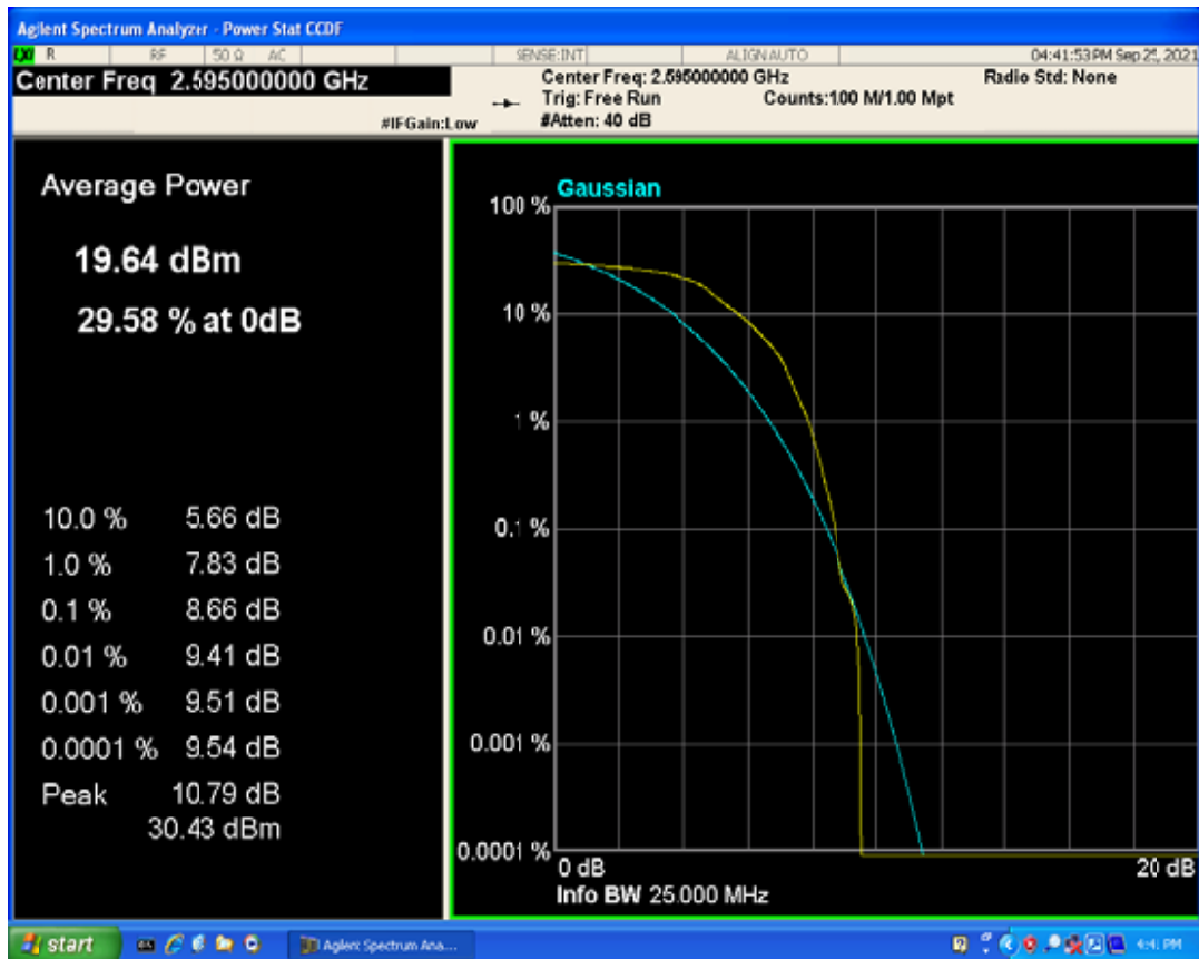
Band5 QPSK BW=1.4MHz Channel=20525 RB Size=1 Position=#0
