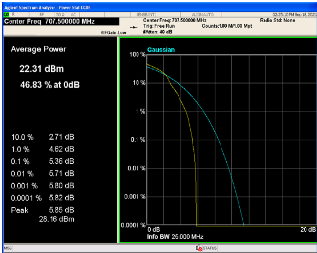
Band12 QPSK BW=5MHz Channel=23095 RB Size=1 Position=#0
