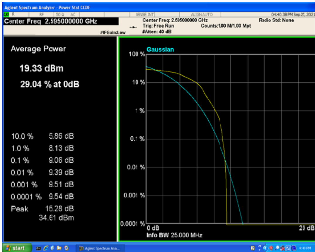
Band41 QPSK BW=10MHz Channel=40640 RB Size=1 Position=#0
