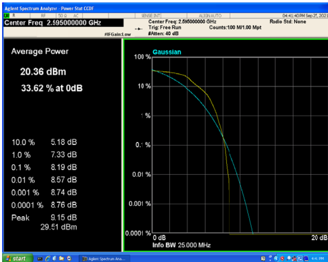
Band41 QAM16 BW=10MHz Channel=40640 RB Size=1 Position=#0
