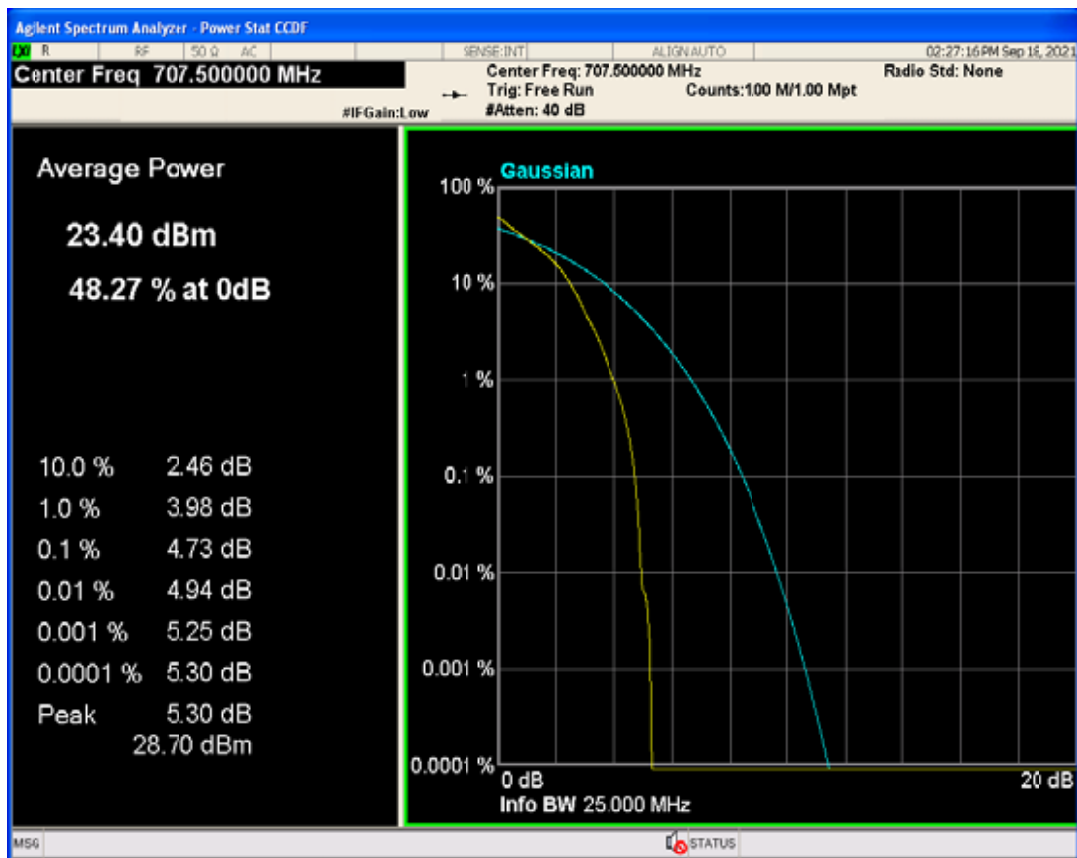
Band12 QAM16 BW=5MHz Channel=23095 RB Size=1 Position=#0
