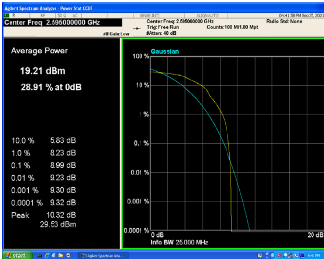
Band41 QPSK BW=20MHz Channel=40640 RB Size=1 Position=#0
