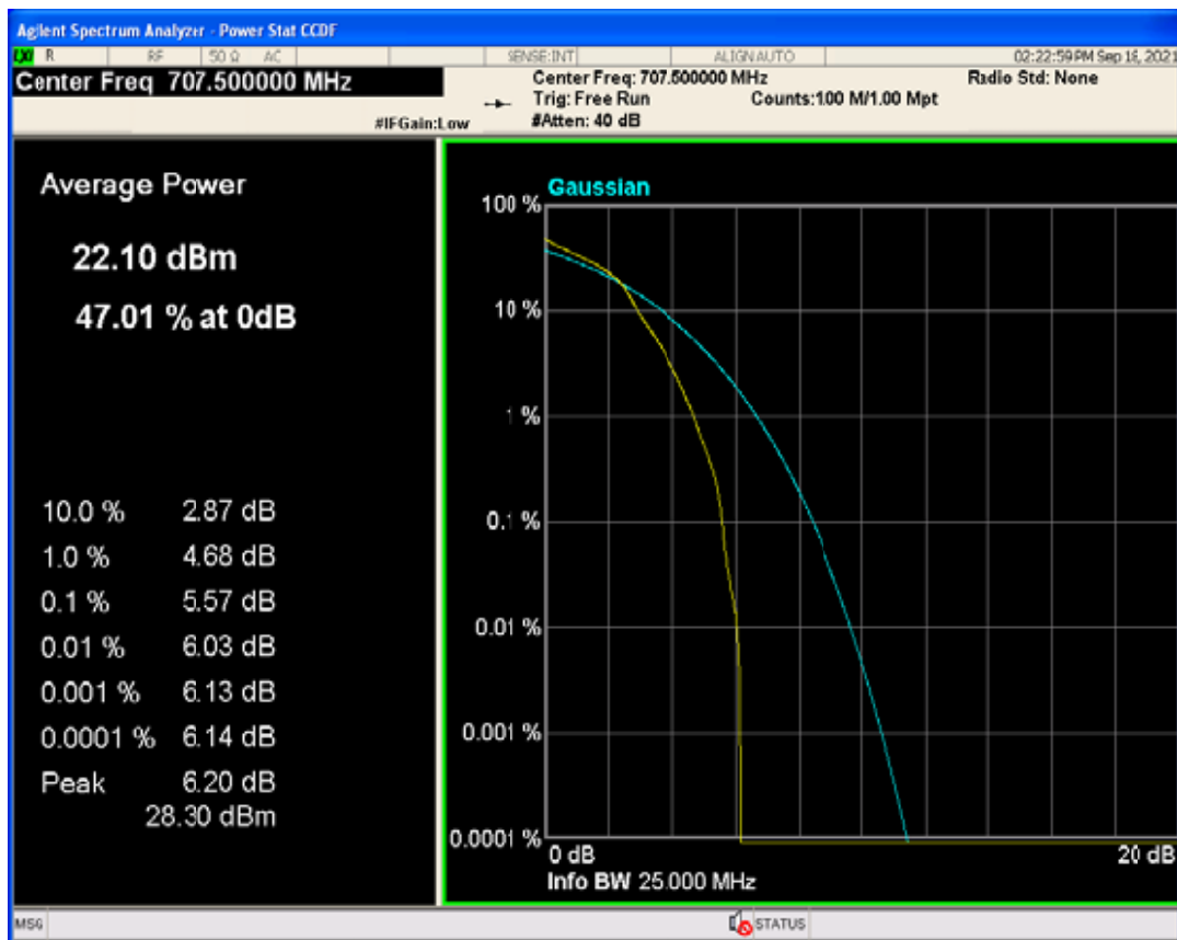
Band12 QAM16 BW=3MHz Channel=23095 RB Size=1 Position=#0
