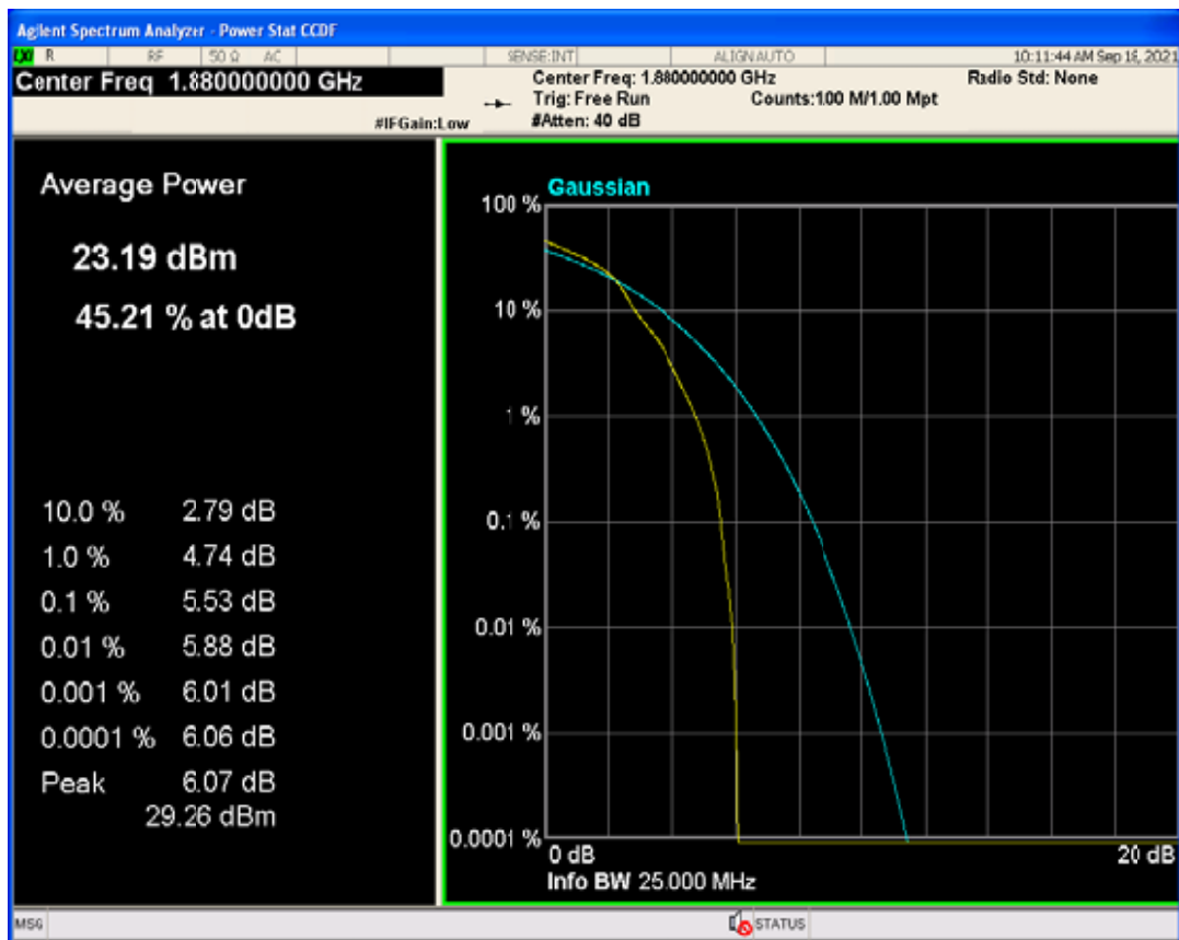
Band2 QPSK BW=15MHz Channel=18900 RB Size=1 Position=#0
