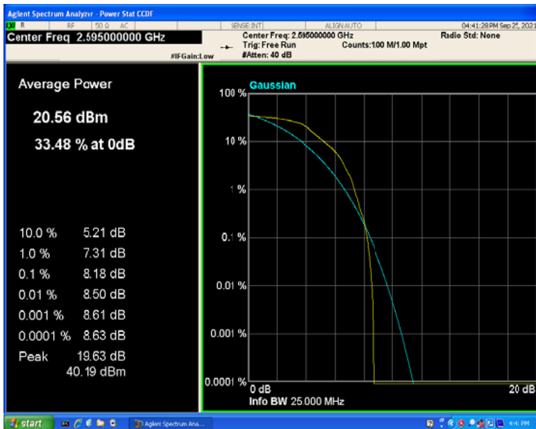
Band41 QPSK BW=15MHz Channel=40640 RB Size=1 Position=#0
