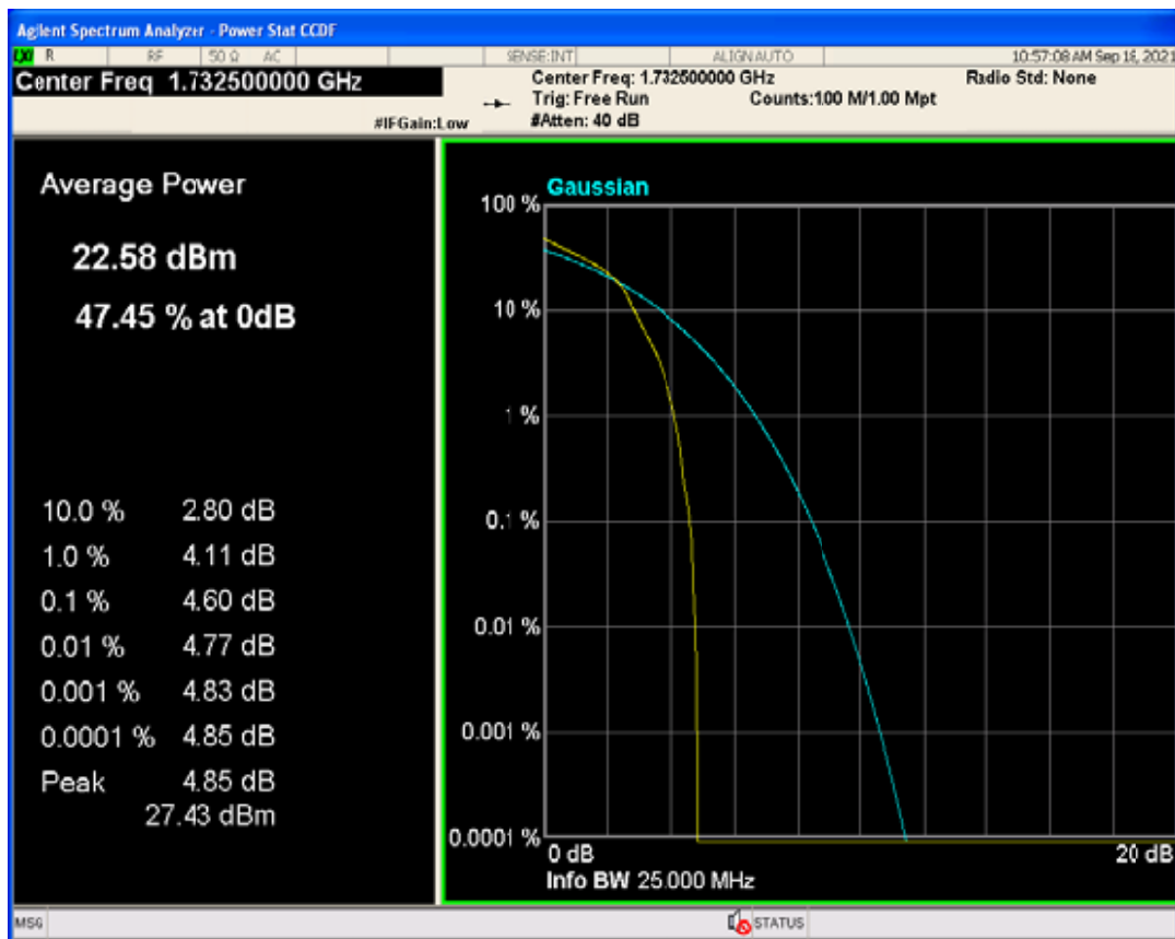
Band4 QAM16 BW=20MHz Channel=20175 RB Size=1 Position=#0
