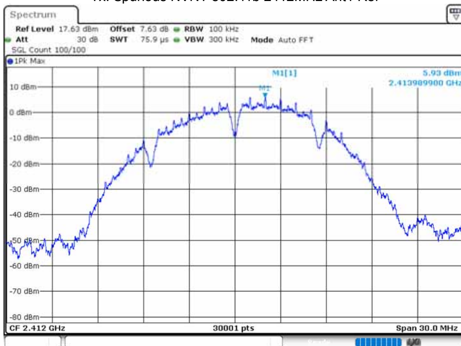
Tx. Spurious NVNT 802.11b 2412MHz Ant1 Ref
