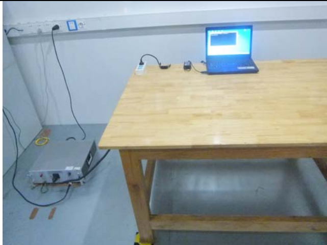
Conducted Emissions Test Setup Front View
