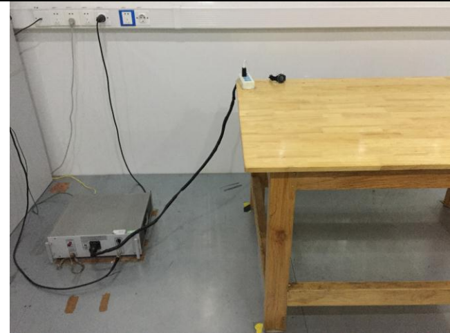
Conducted Emissions Test Setup – Front View
