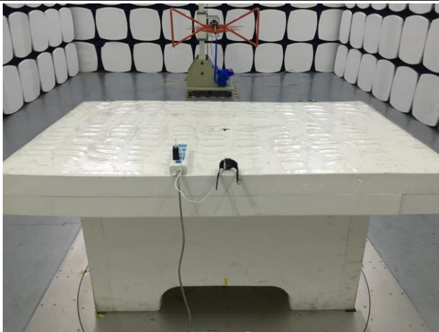
Radiated Emissions Test Setup Below 1GHz
