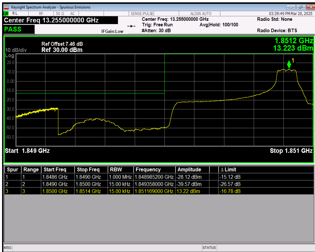
Band2 16QAM BW=1.4MHz Channel=18607 RB Size=6 Position=#0
