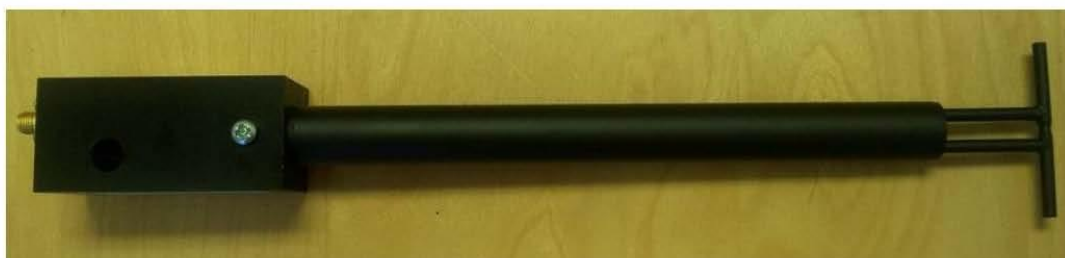
Figure 1 – MVG COMOSAR Validation Dipole
