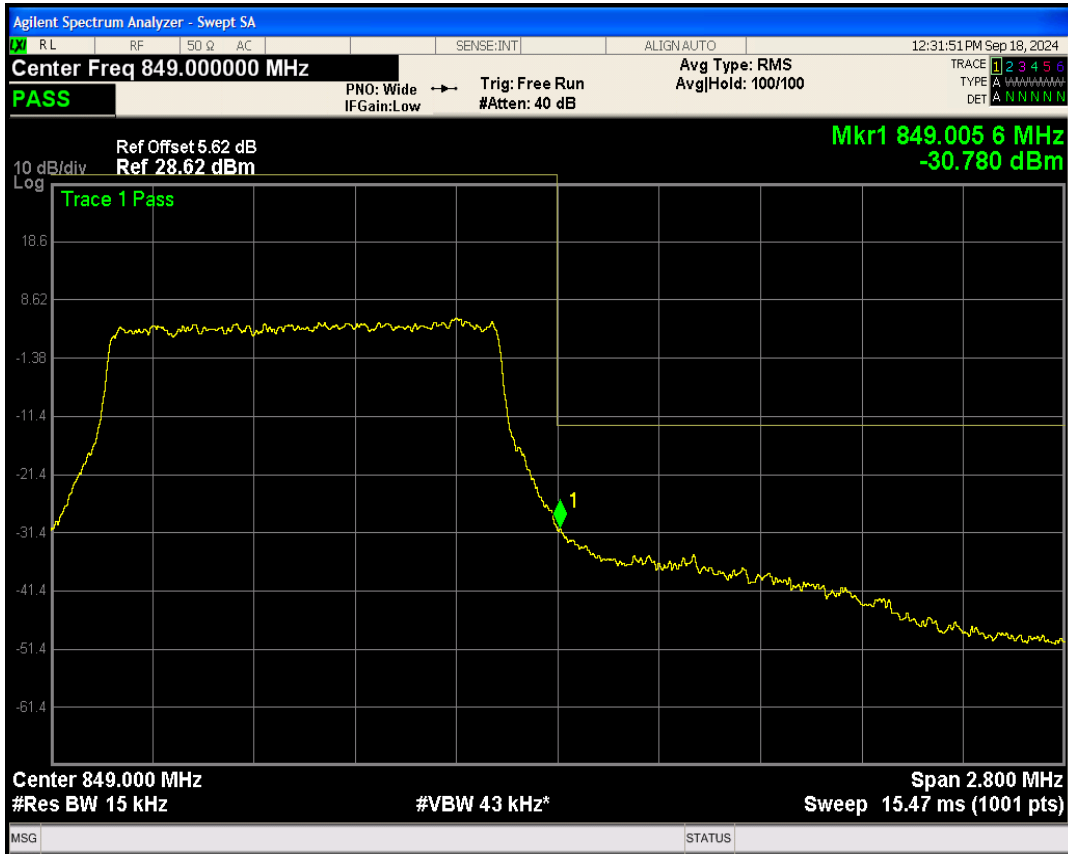
Band5 16QAM BW=1.4MHz Channel=20643 RB Size=6 Position=#0
