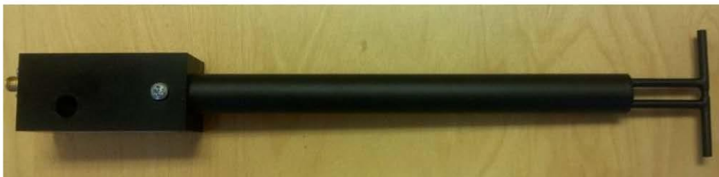
Figure 1 – MVG COMOSAR Validation Dipole
