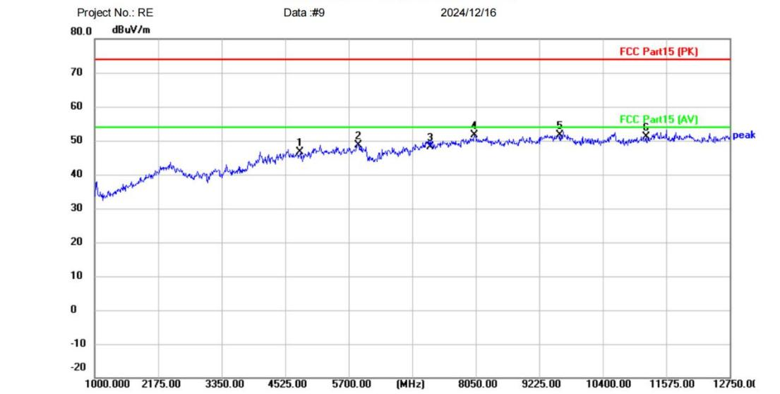
Site: FCC Part15 (PK)      Polarization: **Horizontal**      Temperature: (C)
