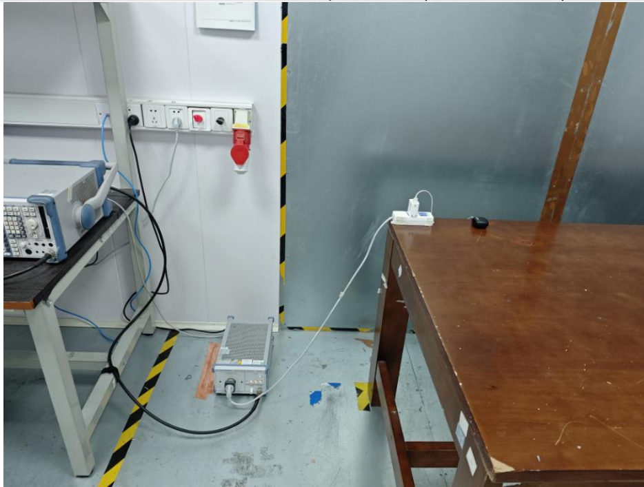
Conducted emissions at AC power line (150kHz-30MHz)
