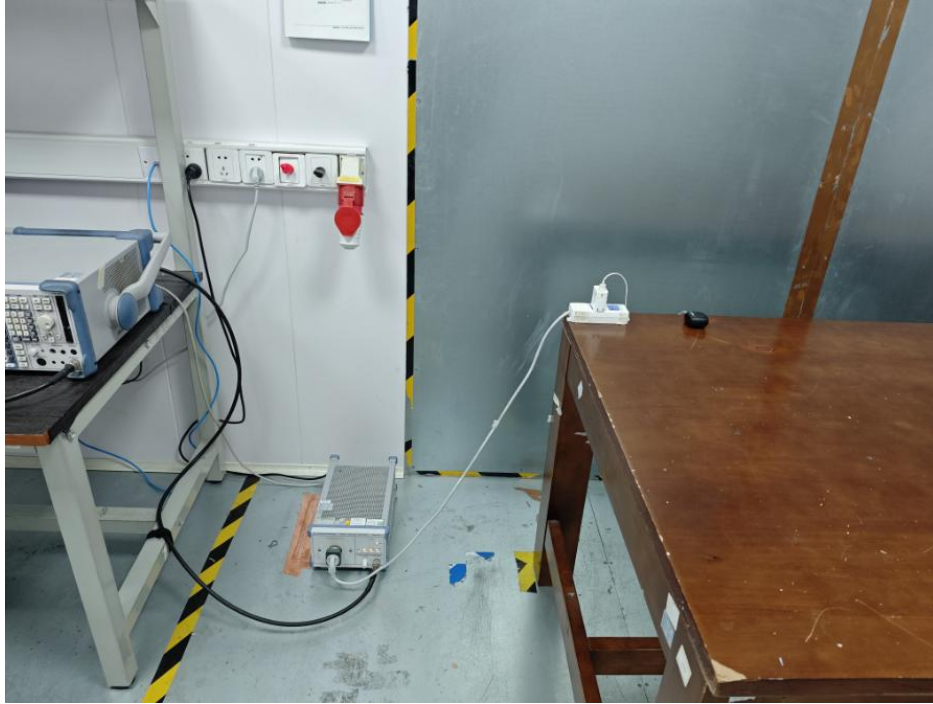
Conducted emissions at AC power line (150kHz-30MHz)
