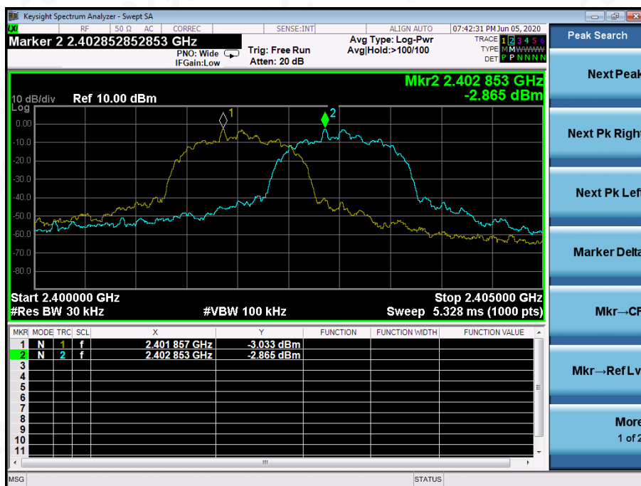
TEST PLOT FOR FREQUENCY SEPARATION
