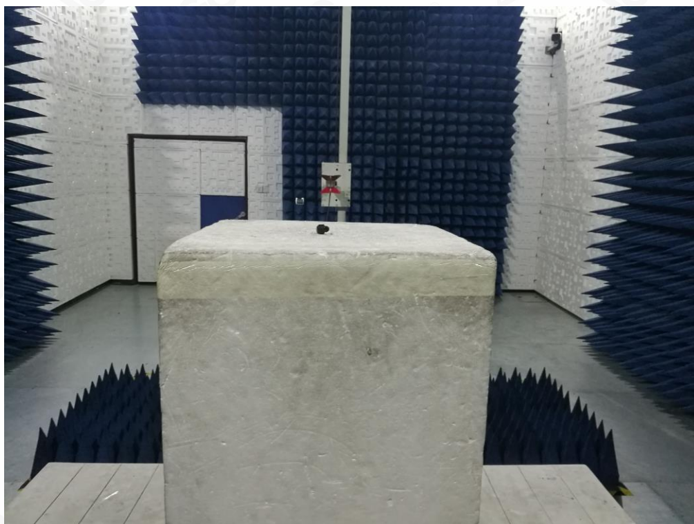
RADIATED EMISSION TEST SETUP ABOVE 1GHZ
