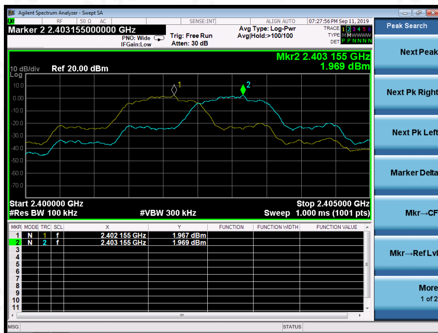
TEST PLOT FOR FREQUENCY SEPARATION
