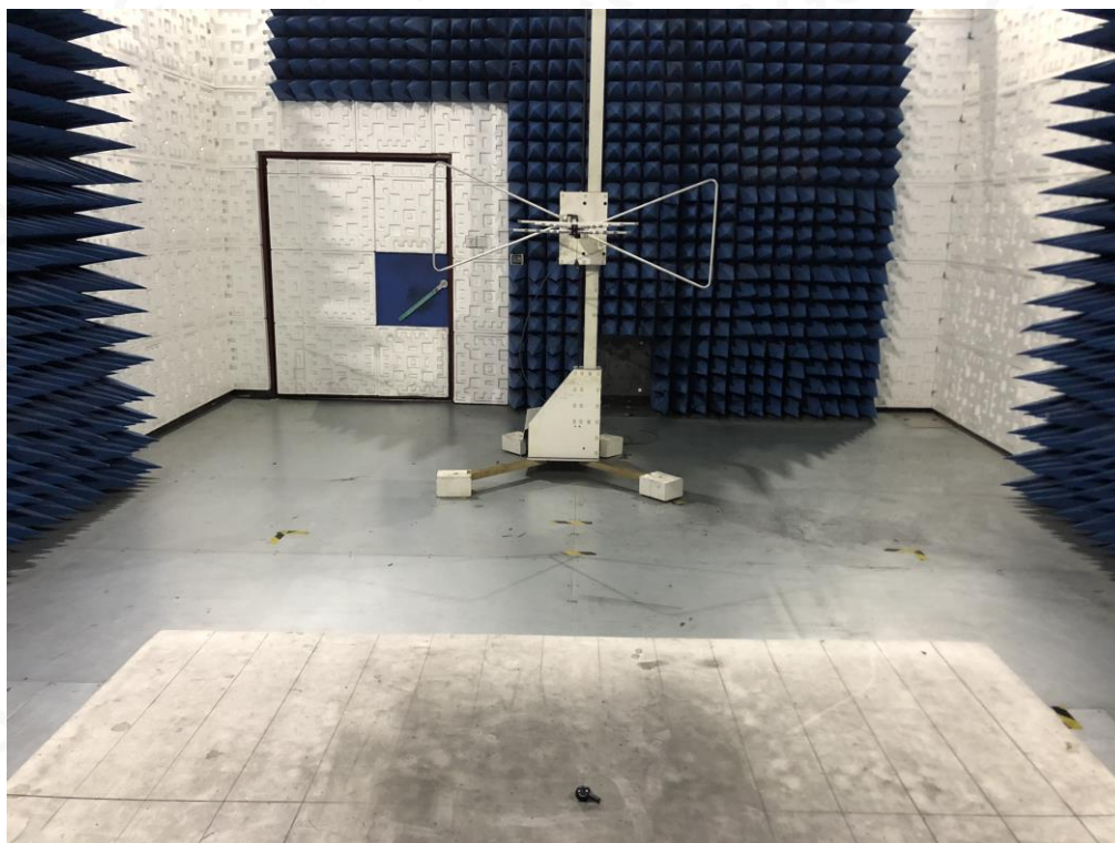
RADIATED EMISSION TEST SETUP ABOVE 1GHZ
