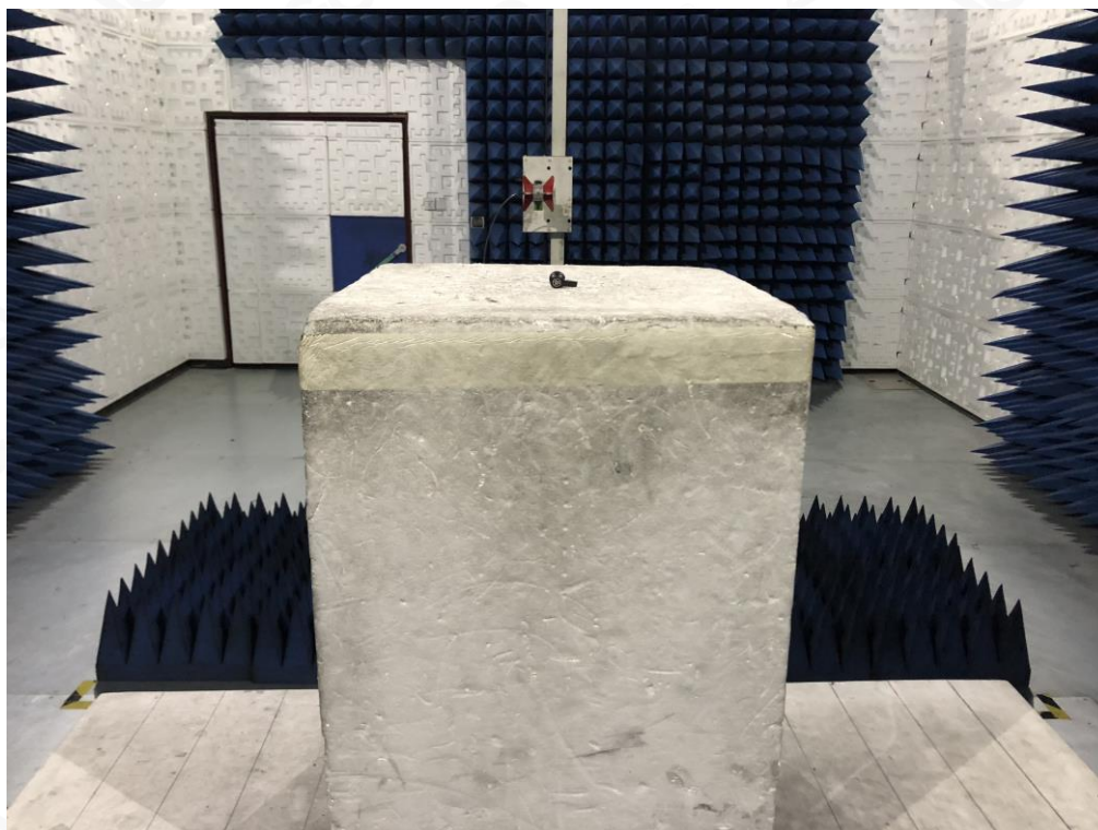
RADIATED EMISSION TEST SETUP ABOVE 1GHZ
