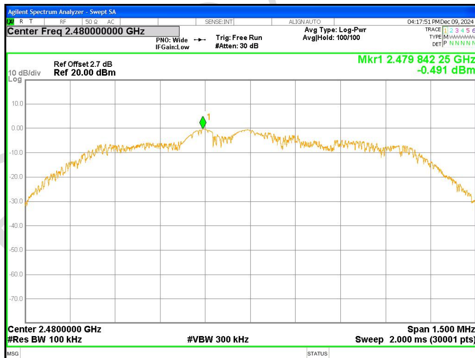
Tx. Spurious NVNT 2-DH1 2480MHz Ant1 Emission
