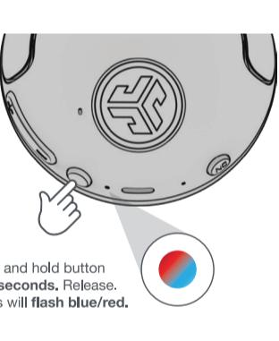
1 Press and hold button for 8 seconds. Release. Lights will flash blue/red.
