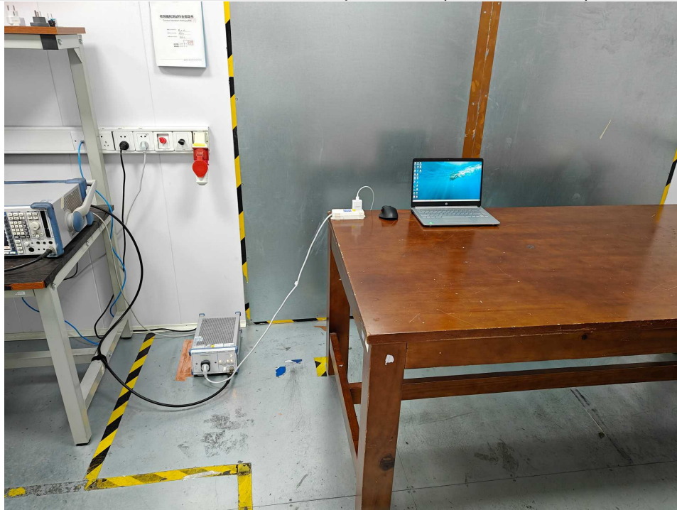
Conducted emissions at AC power line (150kHz-30MHz)
