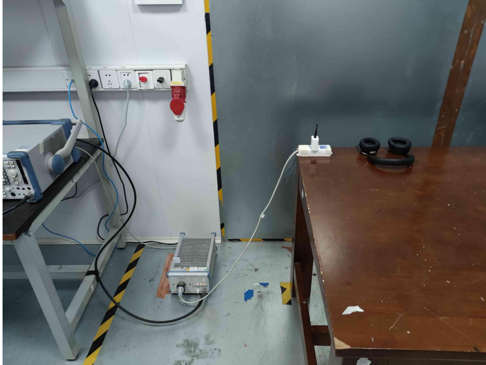
Conducted emissions at AC power line (150kHz-30MHz)
