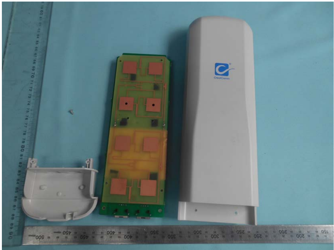
FIGURE 5 INTELLIGENT WIRELESS TRANSMISSION EQUIPMENT (M/N: TB5E) COVER REMOVED
